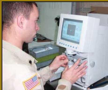
A lensometer is used to measure the power and cylindrical axis of a lens.
