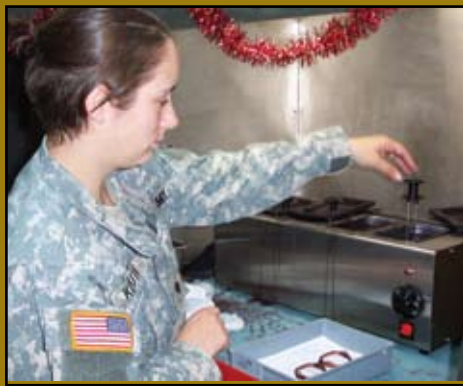
To create sunglasses, lenses are placed into a tint bath until they reach the desired darkness.
