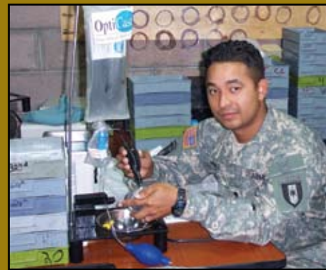
The OptiCast system is used to fabricate bifocals.
