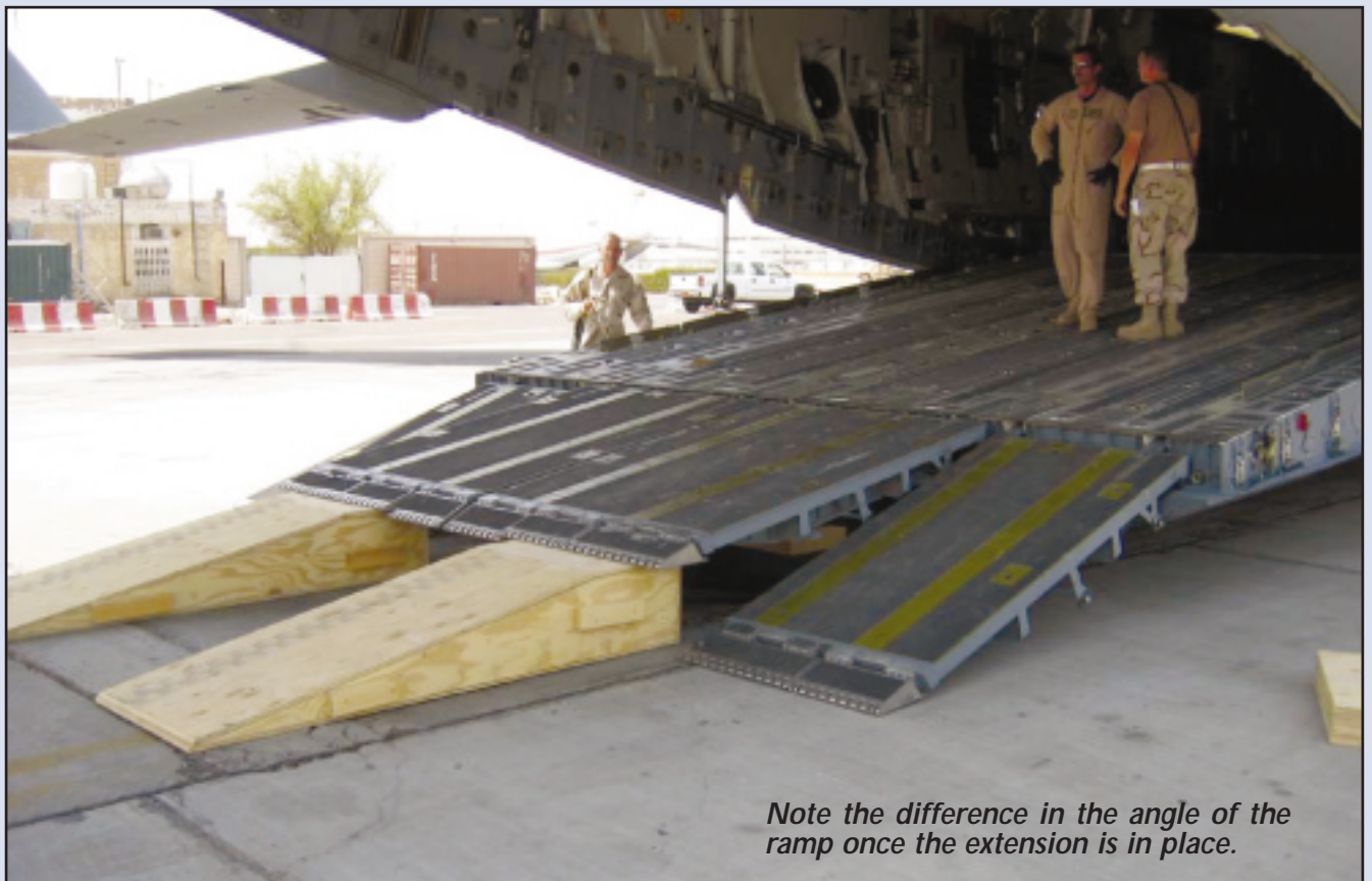
The main ramp pedestal support and two supplemental approach ramps are placed in position for loading the AOAP van aboard a C-17 transport.
