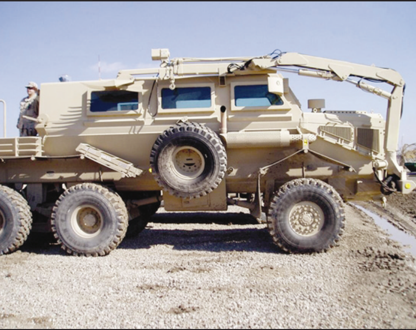
The 23-ton Buffalo is the newest piece of equipment Operation Iraqi Freedom soldiers have to identify improvised explosive devices.
