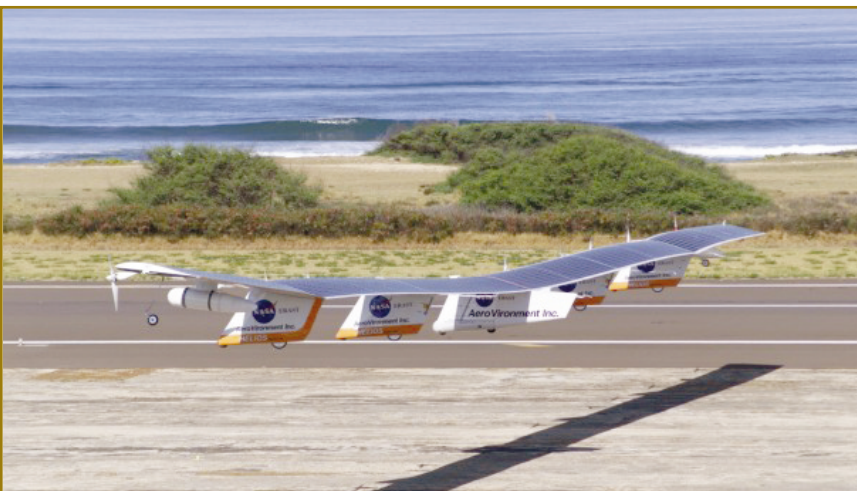
The potential of photovoltaics in transportation was demonstrated by the Helios prototype airplane, which used solar panels to power its electric motors. It was developed by AeroVironment, Inc., of Monrovia, California, for the National Aeronautics and Space Administration.
