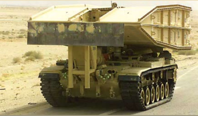
An M60A1 armored vehicle launched bridge carries a bridge to the location where it will be installed.
