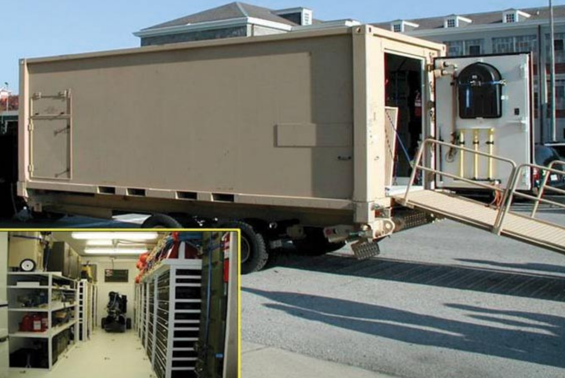
Tools in the Standard Automotive Tool Set (SATS) come stored in a deployable container. The inset shows the storage configuration of the SATS container.
