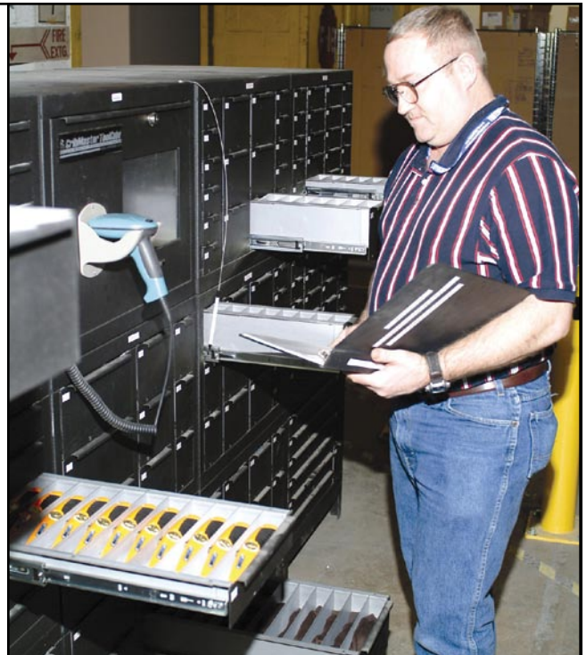
A tool crib parts attendant checks the inventory on the point-of-use vending machine.
