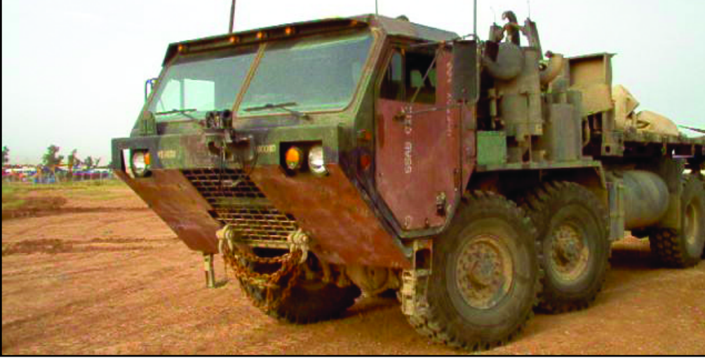
HEMMT armor protects drivers of large transport vehicles.
