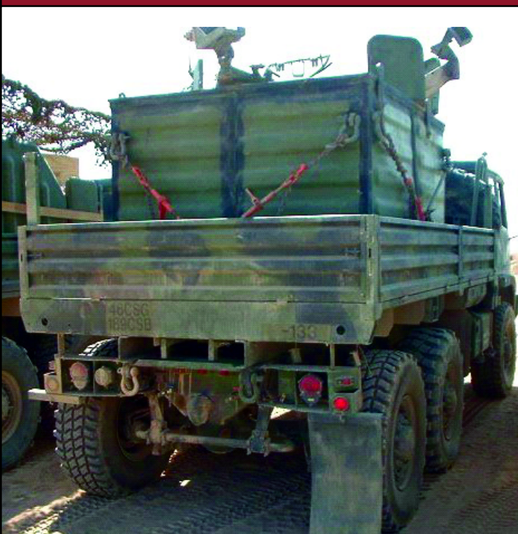
Welders assigned to the 548th Corps Support Battalion during Operation Iraqi Freedom create an armored “box” (above) for positioning in the back of a gun truck. Note the gun mounts on the armored box in the back of the vehicle (below).
