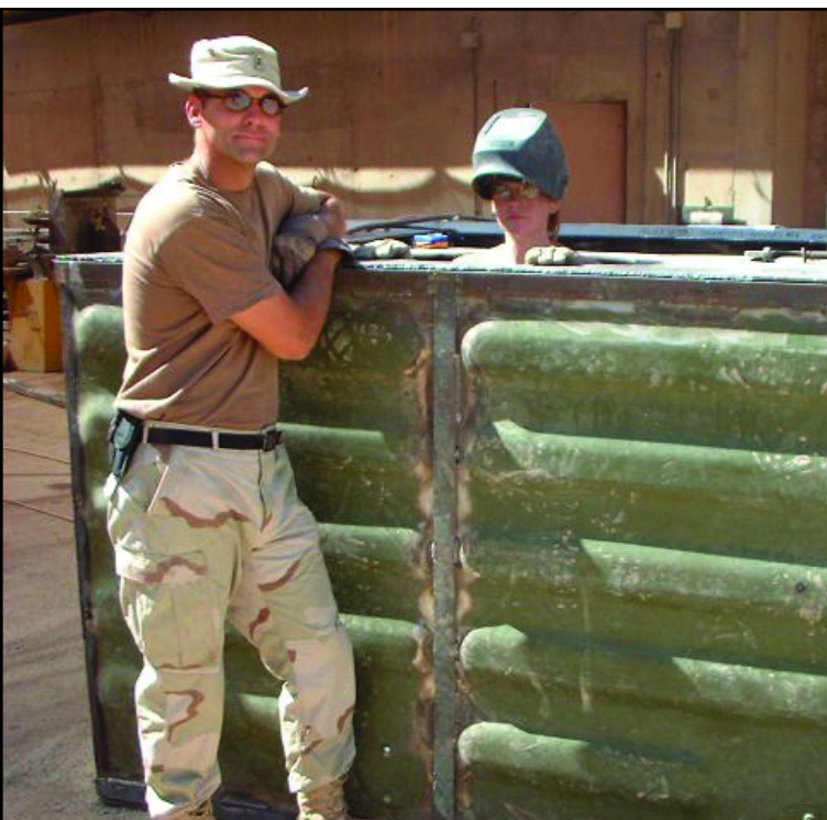
Welders assigned to the 548th Corps Support Battalion during Operation Iraqi Freedom create an armored “box” (above) for positioning in the back of a gun truck. Note the gun mounts on the armored box in the back of the vehicle (below).
