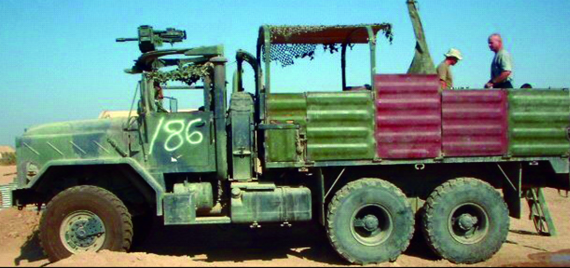
A gun truck is constructed by welding armor plates to the sides of a 5-ton truck. A ring-mounted MK19 40-millimeter machinegun is emplaced in front, and a .50-caliber machinegun is mounted in back.
