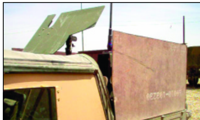
Armor on gun trucks protects the gunner in the back of the truck.
