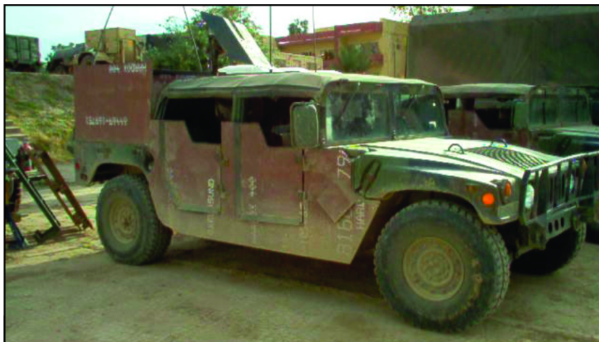
This up-armored HMMWV resembles a Mad Max vehicle, thus the nickname “Mad Attakai” for the name of the welder who designed the armor.
