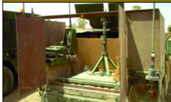
Armor on gun trucks protects the gunner in the back of the truck.
