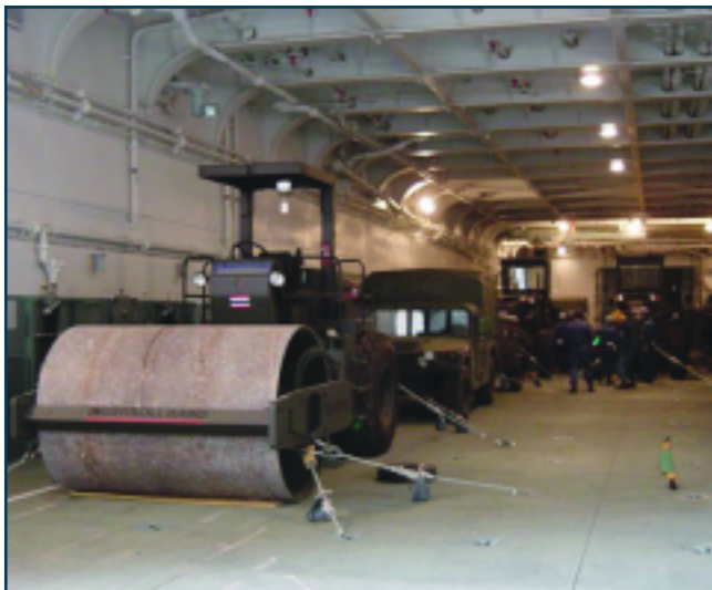
A vibratory roller is tied down inside the ship.
