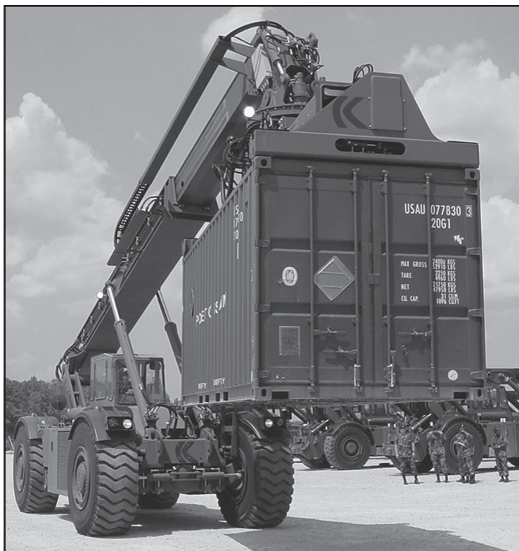
□ The RTCH-240 can rotate a container 180 degrees with its boom and can stack containers three high.
