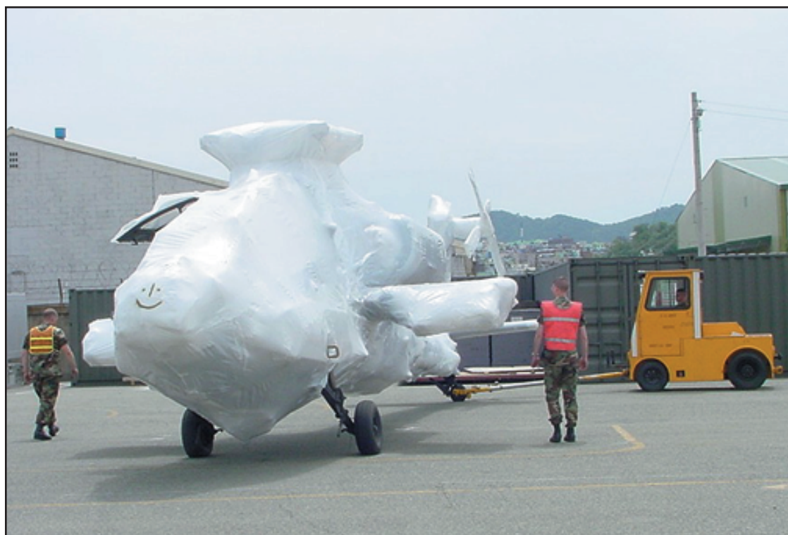
□ A shrink-wrapped helicopter is towed to the MS Green Dale for loading.
