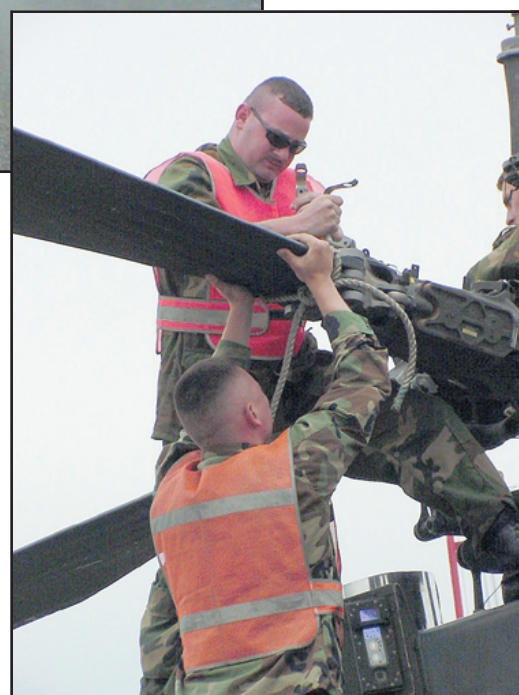
Chemical specialists from the 61st Chemical Company, 23d Chemical Battalion, spray a helicopter with freshwater to wash away salt deposits. Below, crowning straps are removed from the rotor blades of an Apache by soldiers from G Company, 52d Aviation Regiment.
