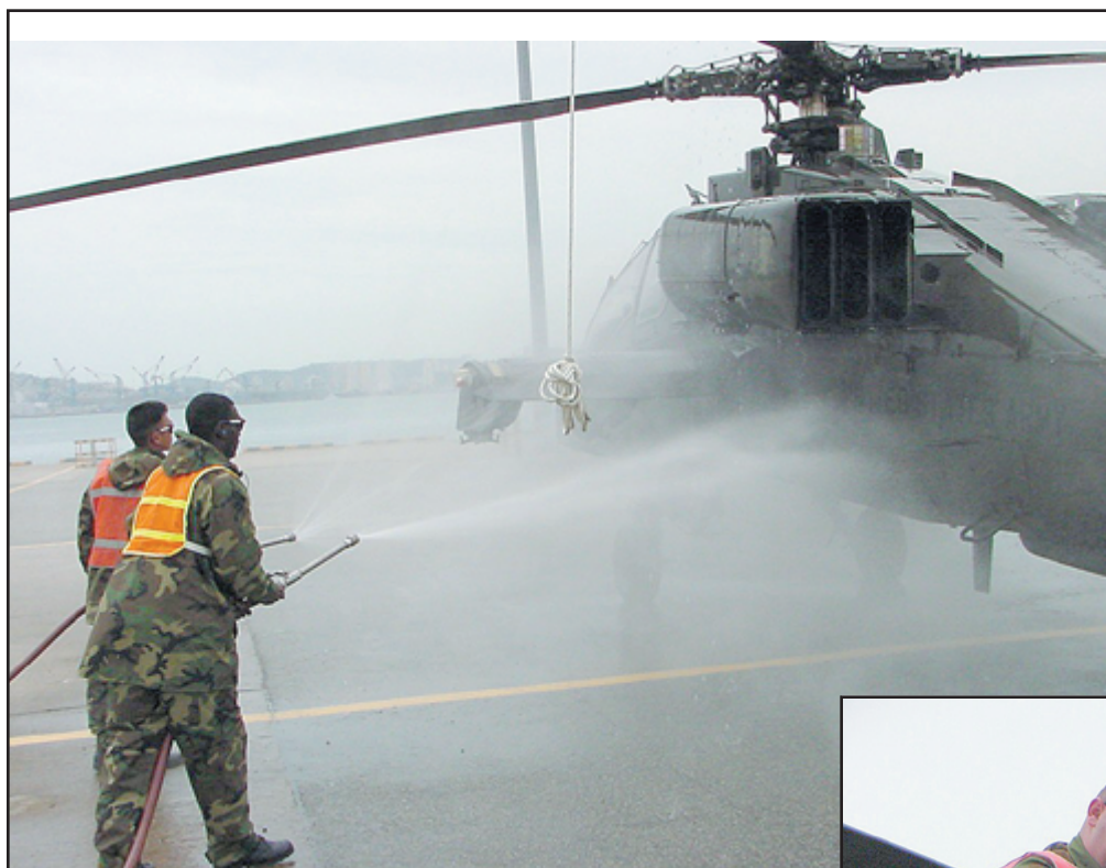
Chemical specialists from the 61st Chemical Company, 23d Chemical Battalion, spray a helicopter with freshwater to wash away salt deposits. Below, crowning straps are removed from the rotor blades of an Apache by soldiers from G Company, 52d Aviation Regiment.
