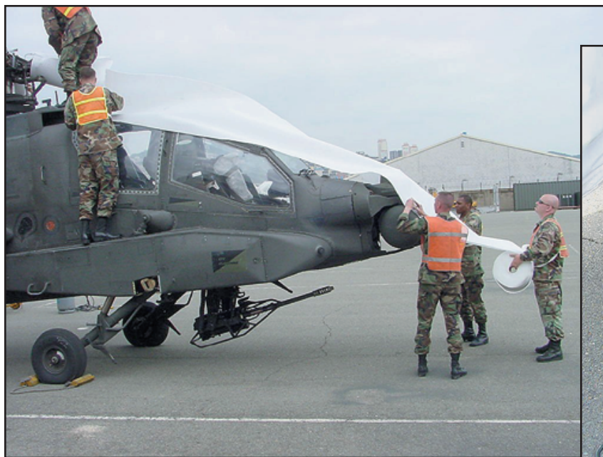
□ Above, an Apache helicopter is covered with plastic wrap to protect it from the salt spray. At right, a G Company soldier applies heat to the plastic wrap to shrink it tightly over the aircraft.
