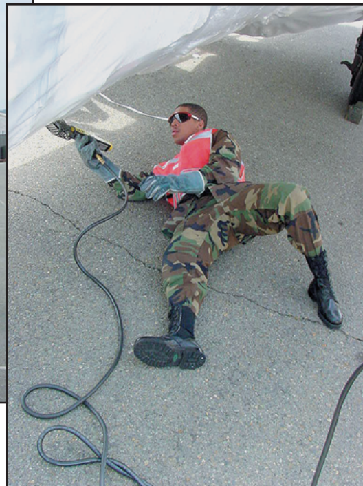
□ Above, an Apache helicopter is covered with plastic wrap to protect it from the salt spray. At right, a G Company soldier applies heat to the plastic wrap to shrink it tightly over the aircraft.
