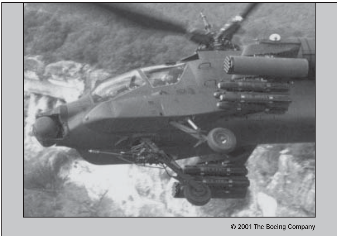
□An AH-64 Apache helicopter loaded with 8 Hellfire missiles and 19 rockets maneuvers to the objective.
