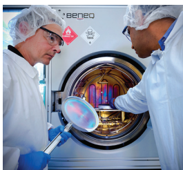
Goddard technologist Vivek Dwivedi (right) and his University of Maryland collaborator, Raymond Adomaitis (left), are shown here with a sample and the reactor that they will use to apply thin films onto the substrate using atomic layer deposition.
