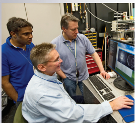
The Visible Nulling Coronagraph combines an interferometer with a coronagraph to image and characterize Jovian-size planets. In this photo, Principal Investigator Rick Lyon (foreground), Udayan Mallik (left), and Sigma Space's Pete Petrone (right) are monitoring the progress of wavefront control using the technology, which is operating inside a vacuum tank. (Photo Credit: Chris Gunn)
