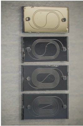
This photo shows examples of four different lengths of the microchannel component that is at the core of Principal Investigator Stephanie Getty's "lab-on-a-chip" liquid chromatograph. Getty is developing the technology under NASA follow-on funding to detect and analyze organic compounds, including amino acids. (Photo Credit: Chris Gunn)
