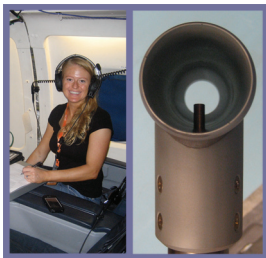
University of Maryland graduate student Heather Arkinson monitored the IRAD-funded In-Situ Airborne Formaldehyde Instrument. The image on the right shows the new air-sampling system that more efficiently draws in air and prevents particles from contaminating formaldehyde measurements.
