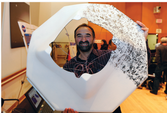
Engineer Ken Segal, who has been instrumental in promoting the use of composites in spacecraft design, holds the upper skin of a telescope housing made entirely of composite materials. The structure was originally designed for the Tropospheric Wind Lidar Technology Experiment, an instrument that could fly next year as part of NASA’s Hurricane and Severe Storm Sentinel mission.
