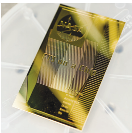
ABOVE: George Shaw (left), Shahid Aslam (center), and Tilak Hewagama (right) are testing their spectrometer-on-a-chip (LOWER) that could dramatically reduce the size of future instruments. (Photo Credit: Chris Gunn)
