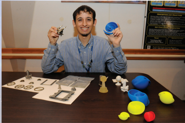
No, these aren't toys. Principal Investigator Steven Kenyon created these devices using an emerging technology called "Direct Metal Laser Sintering." With this 3-D manufacturing process, engineers and scientists may be able to fabricate novel instruments considered impractical or even impossible before. In his right hand, Kenyon holds a modulated X-ray source; in his left, a 3-D representation of the magnetic field emanating from a pulsar.
