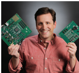
Jonathan Pellish holds in his right hand a Goddard-developed digital test board. In his left is the IRAD-developed daughter card containing the analog-based data-processing integrated circuit. The daughter card snaps into the digital test board and will be used to test a number of spaceflight-processing applications.
