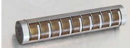
This is a prototype EHD pump that Principal Investigator Jeffrey Didion validated during a flight experiment in 2012. (Photo Credit: Chris Gunn)
