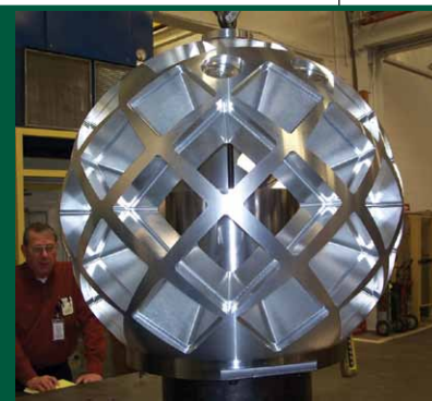
Fig. E2. Detector array for the MaNDi instrument.
