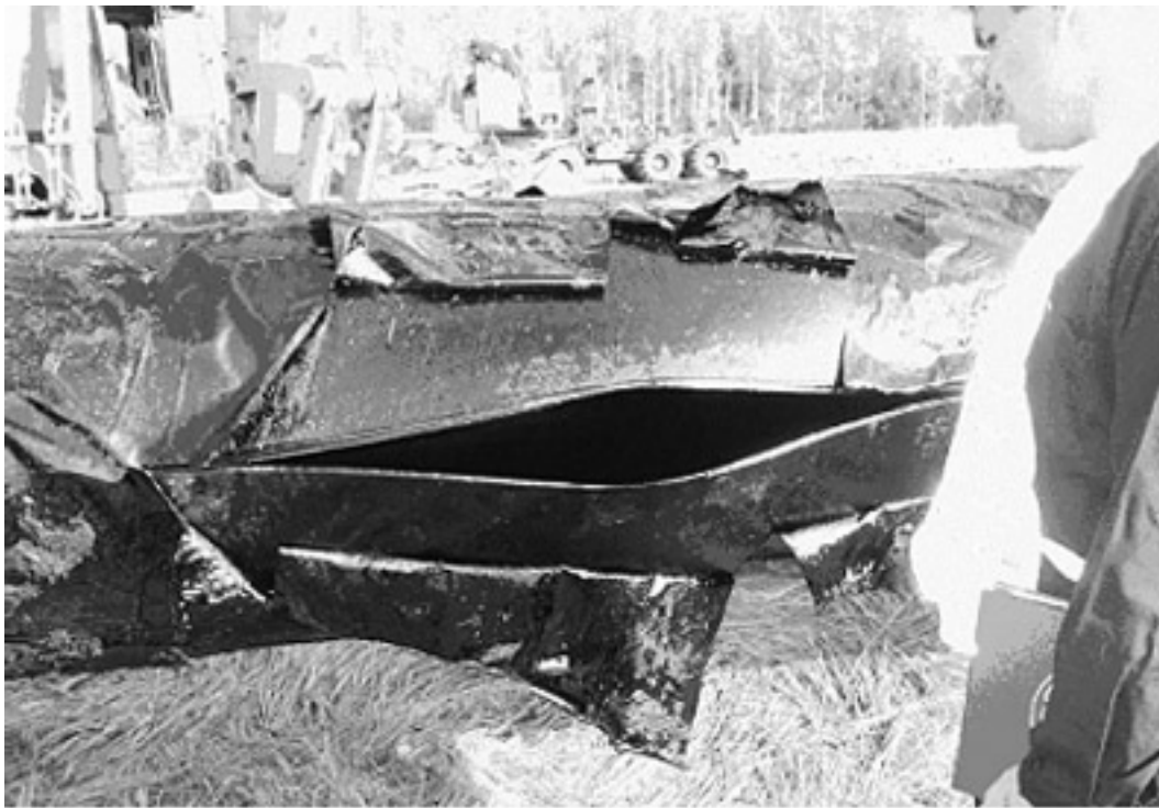
Ruptured pipeline section of the 34" line.
