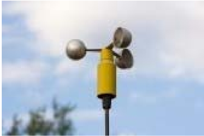
An anemometer, which measures wind speed
