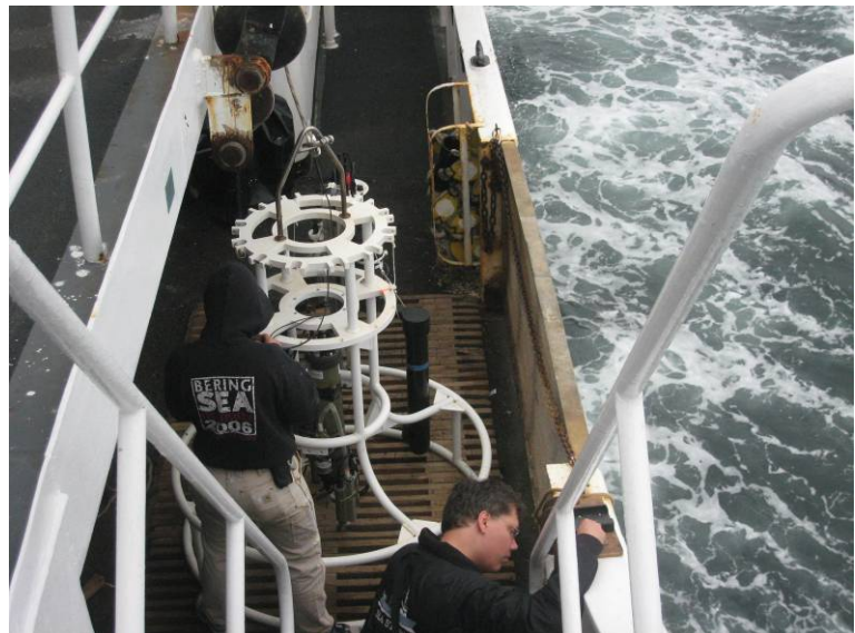
The CTD, resembling a giant wedding cake constructed of painted steel, measures the composition of the water, salinity, temperature, oxygen levels, and water pressure.
