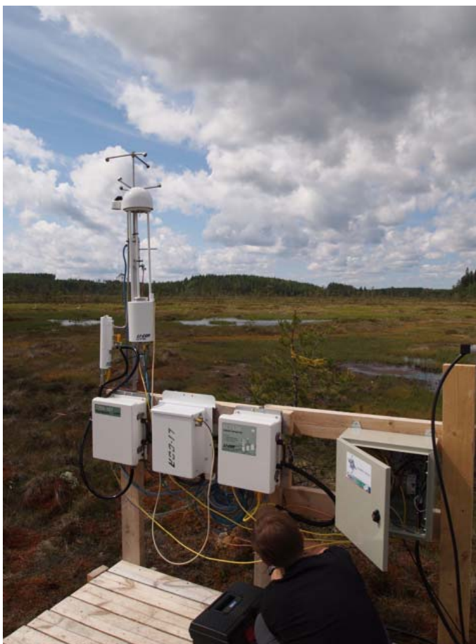
Figure 1: Sami Haapanala installing the measurement systems at the ombrotrophic Siikaneva II site. This site is run by batteries, and is charged from time to time by a diesel generator.
