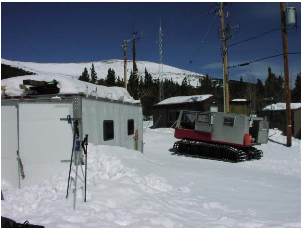
Figure 2: Conducting winter flux research at the C1 NOAA site. The trailer in the foreground houses the computers and other equipment for the Niwot Ridge AmeriFlux tower.
