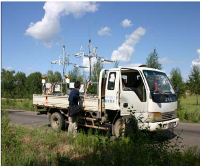
Photo 2: The mobile J-Rovers deployed on the Mongolia Plateau in 2009. These towers are moved across the plateau annually to gain information of as many ecosystems as possible for regional estimates of carbon and water fluxes through scaling up exercises.
