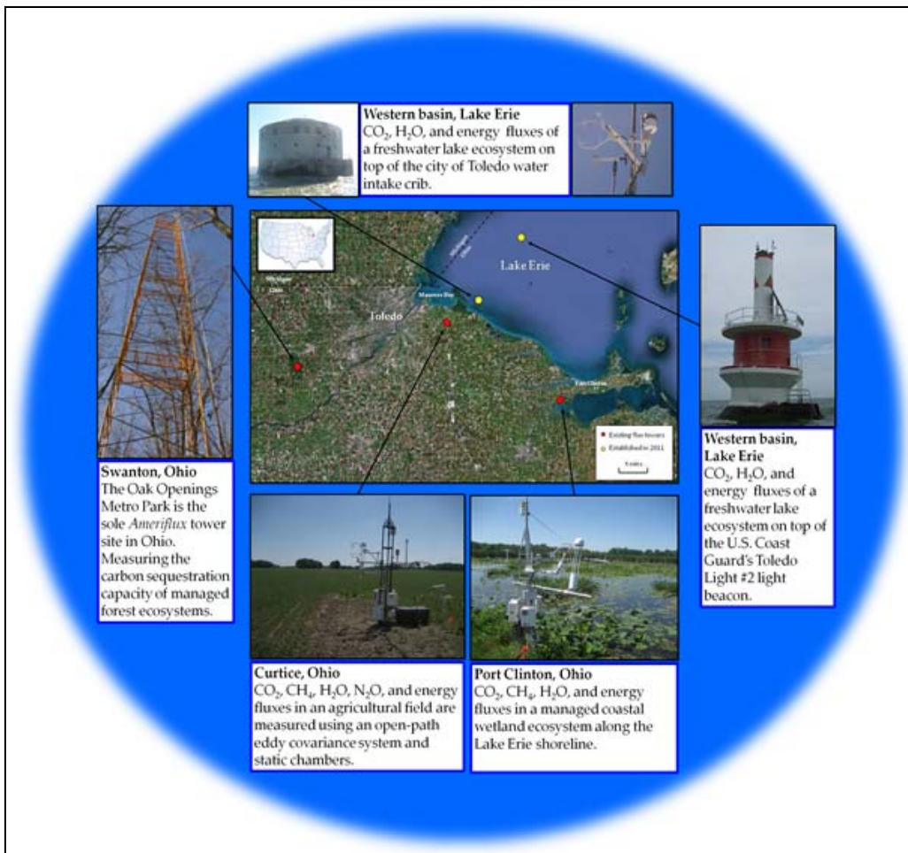
Photo 3. The environmental sensor network (ESN) at the western Lake Erie Basin. The tower cluster is the foundation for basic scientific investigations, education, and policy making through the Lake Erie Center, University of Toledo.
