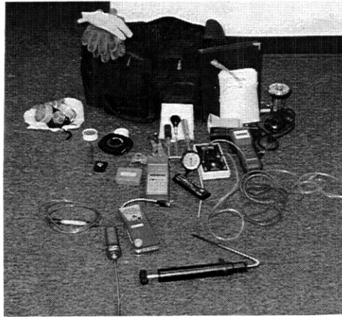
Fig. 2.2. Weatherization Coalition auditors in New York City must pack their tools of the trade in a container suitable for transport on the subway. This kit contains thermometers, a combustibile gas sensor, a combustion analyzer, a CO sensor, a CO sensor, a draft gauge, and a digital pressure sensor, plus sundry hand tools, tape measures, lights gloves, and safety equipment
