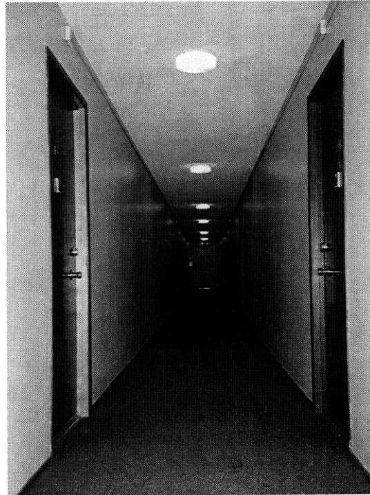
Fig. 6.18. The interior doors are weatherstripped to provide thermal and sonic isolation. The energy-efficient lighting fixtures are cost effective since they are on 24 hours a day.
