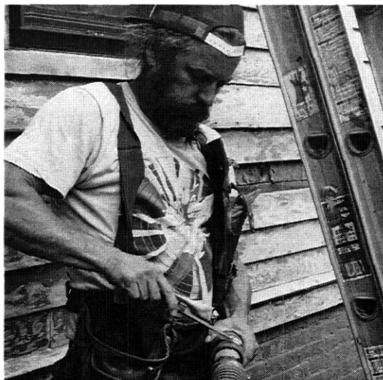
Fig. 3.10. Bill Kelly unclogs a blowing tube, a tedious job that must be done quickly to avoid slowing production.
