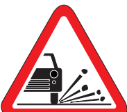
A17 Loose chippings
