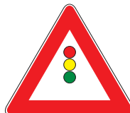
A33 Traffic signals
