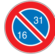
E7 No parking from 16th to the end of the month on this side of the road
