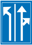
F13 Traffic sign indicating that ahead there are traffic arrows on the road and you must choose a traffic lane
