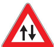
A39 Two-way traffic after a road section with one-way traffic
