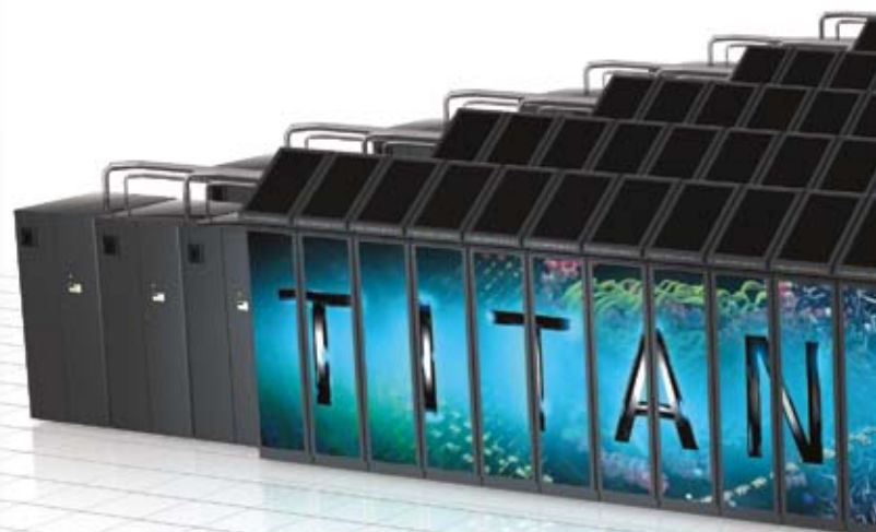
Titan will be capable of performing 20,000 trillion calculations every second, making it six times more powerful than ORNL's current Jaguar system. Image: Andy Sproles
