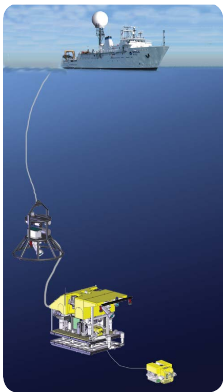
The bell-shaped camera sled, the science-class ROV and the small xBot can operate as deep as 6000 meters. NOAA illustration with vehicle drawings by ROV builder Phoenix International.
