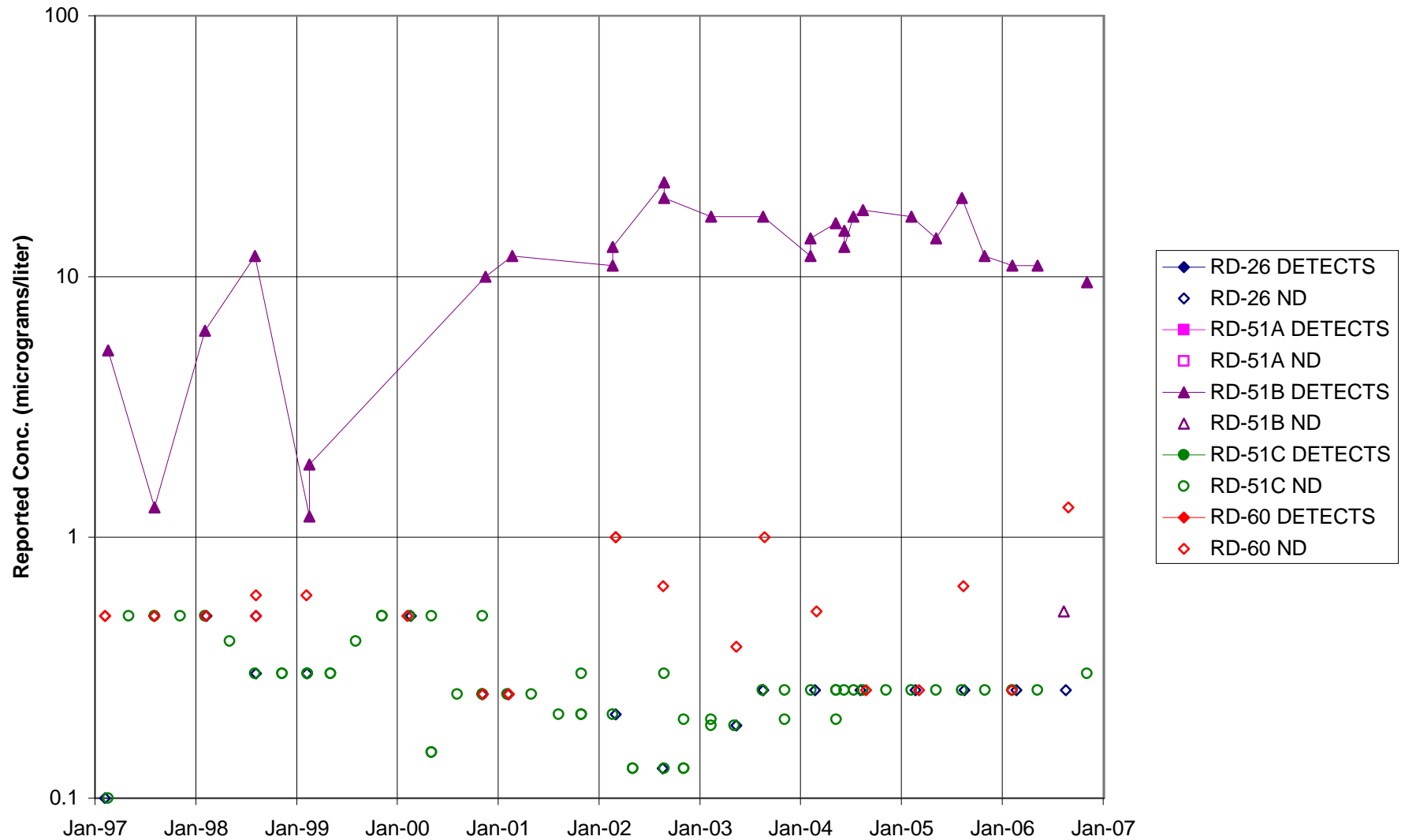
FIGURE F-365. VINYL CHLORIDE in HELIPORT, B/204 AREA WELLS
