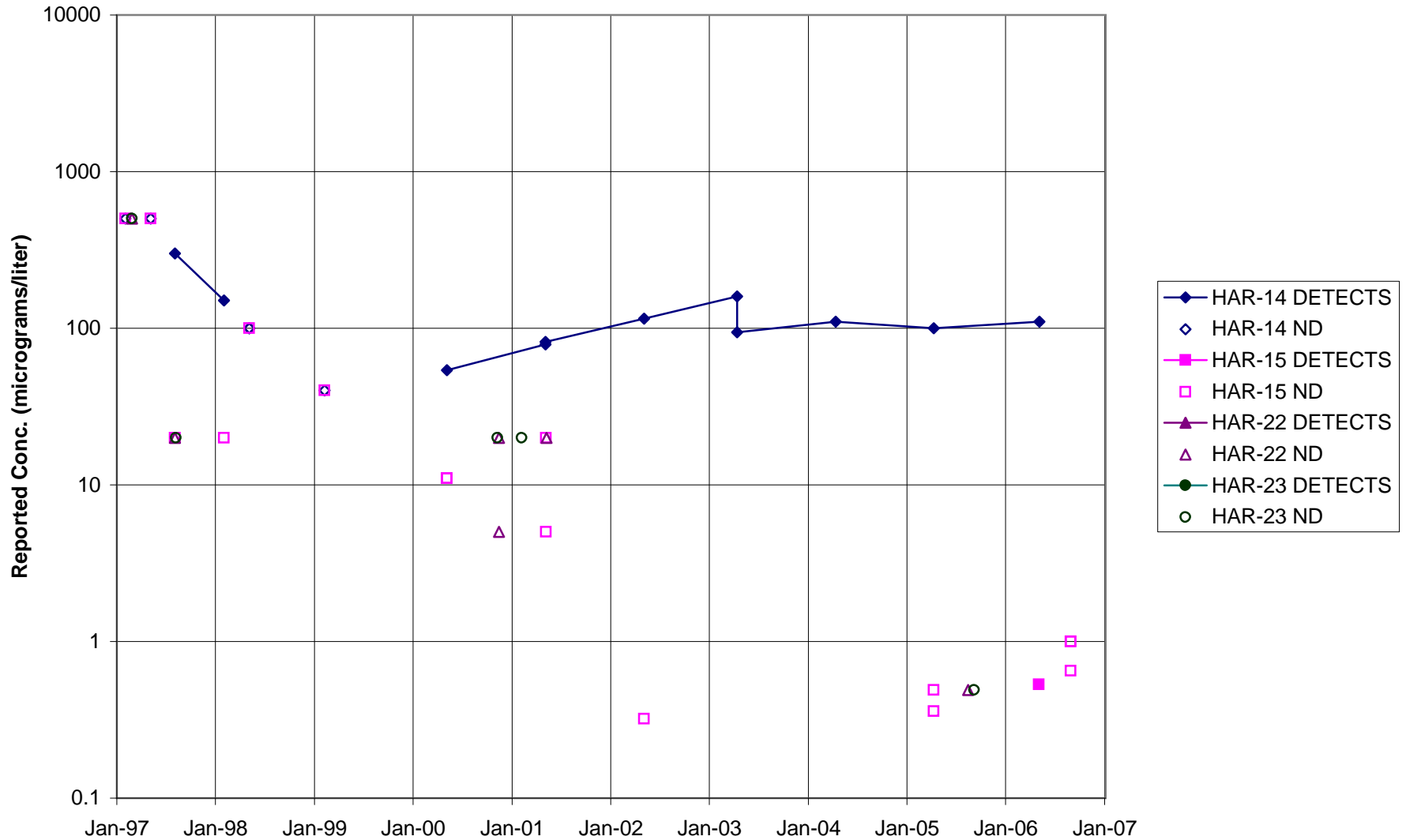
FIGURE F-99. 1,4-DIOXANE in SPA AREA WELLS
