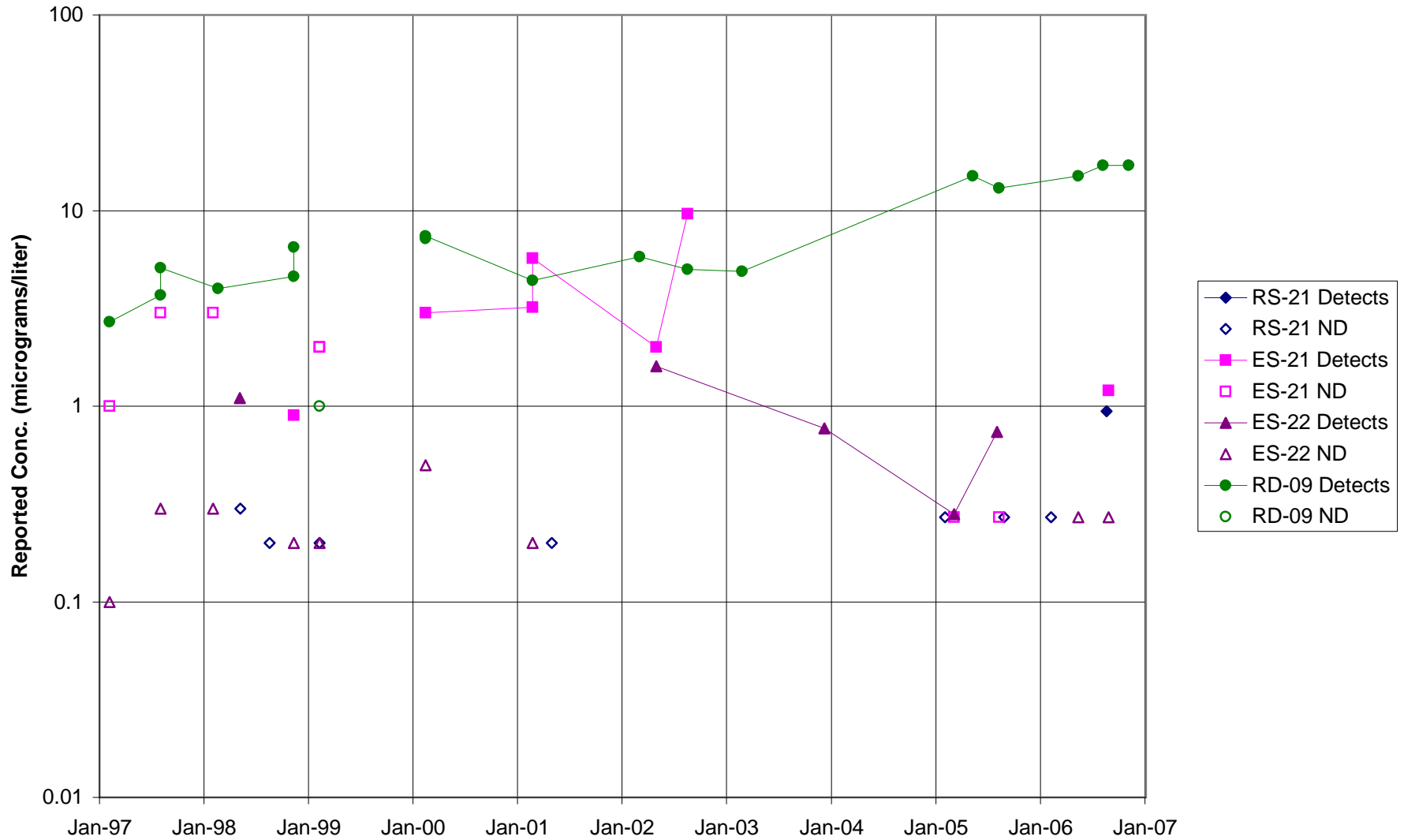
FIGURE F-330. TRANS-1,2-DCE in RD-09 AREA WELLS
