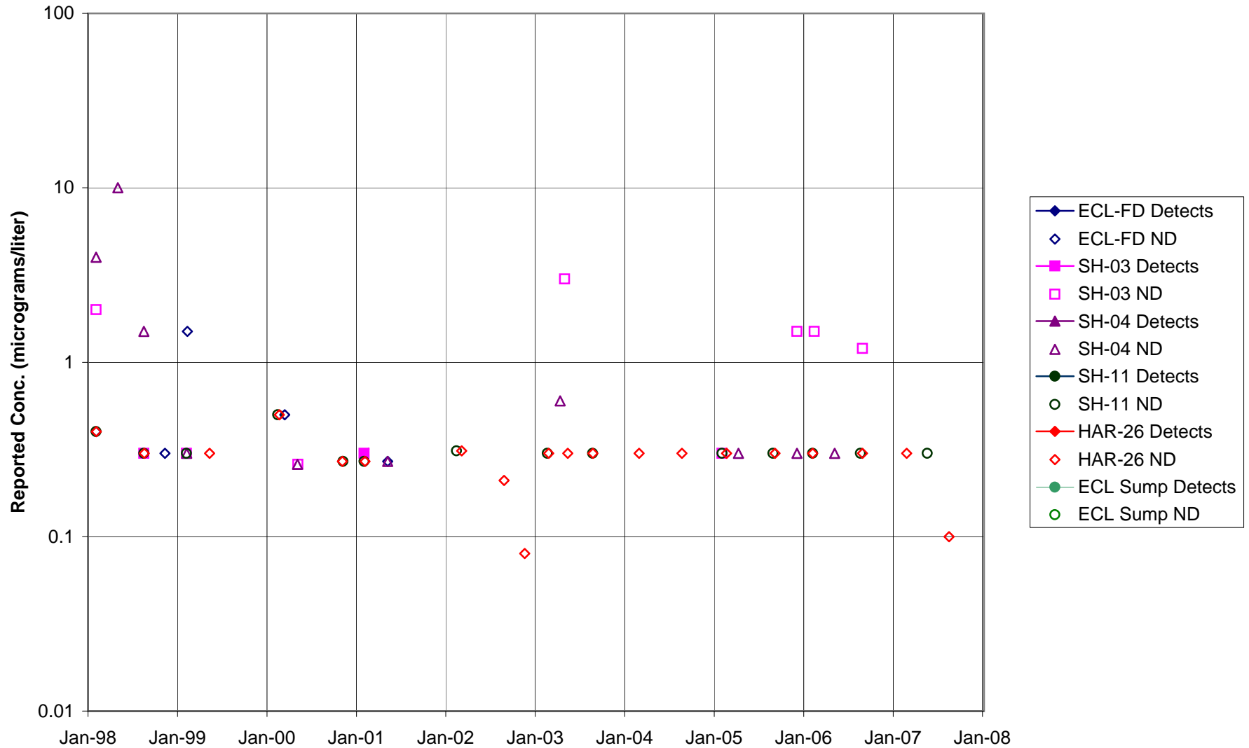
FIGURE F-26. 1,1,2-TCA in ECL AREA WELLS
