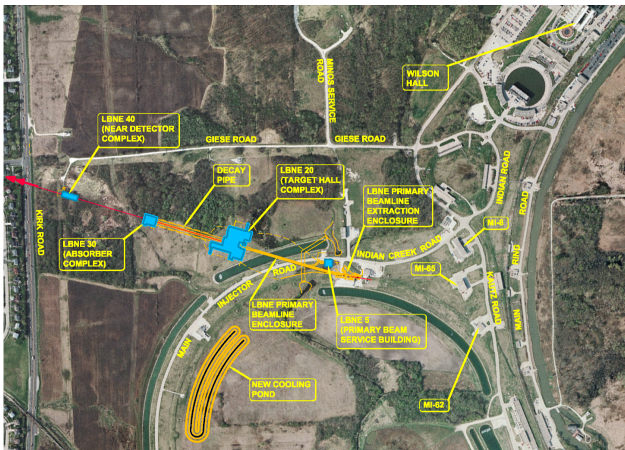
Figure 5-3: LBNE overall project Layout at Fermilab
