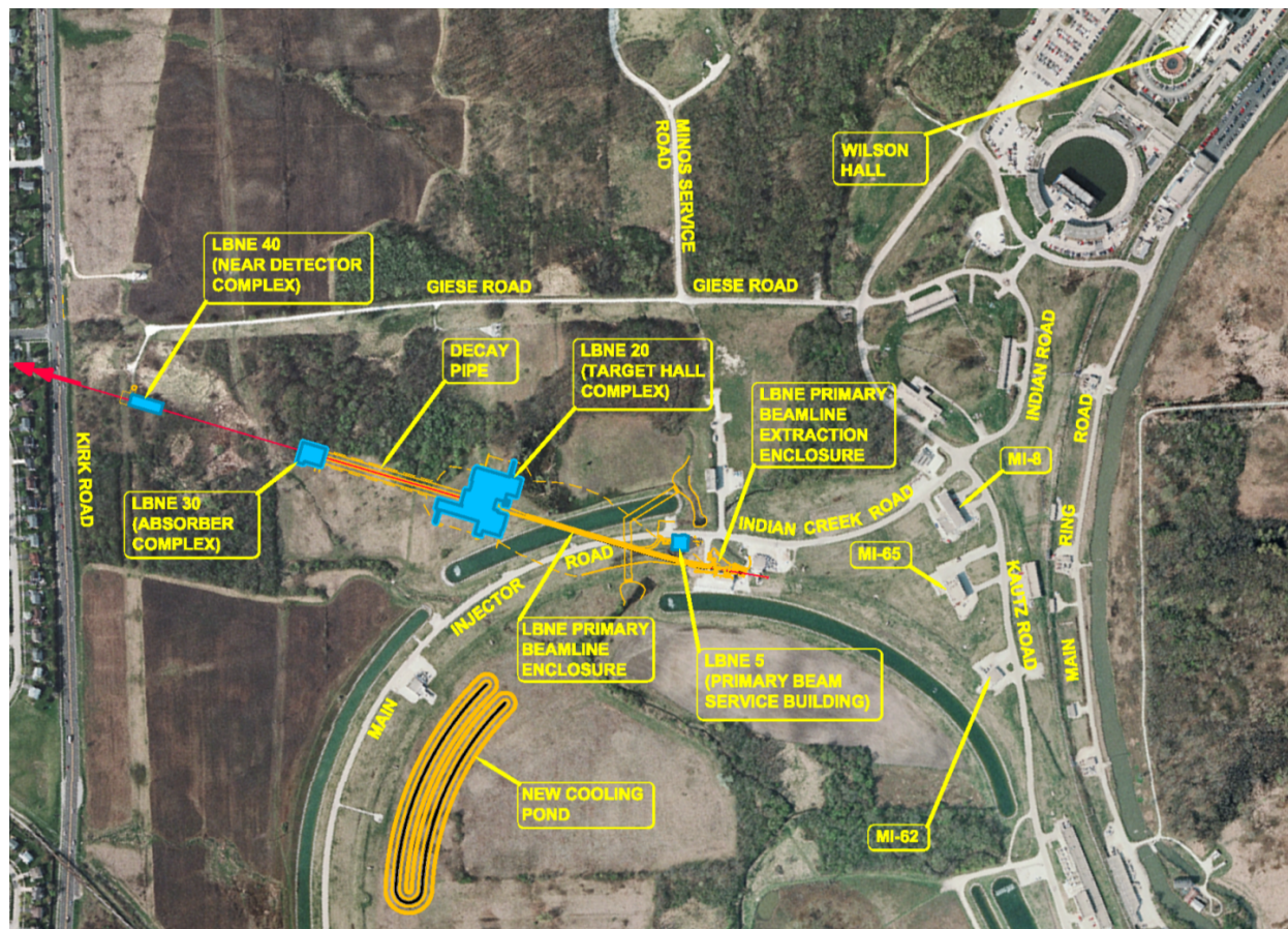
Figure 1-7: LBNE Overall Project Layout at Fermilab
