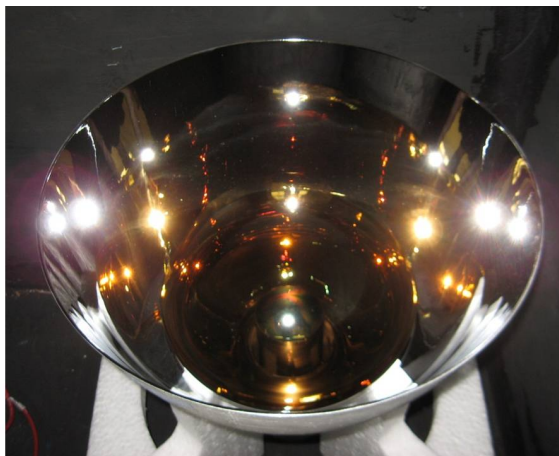
Figure 3–24: Prototype Winston cone mounted on a 10" PMT.
