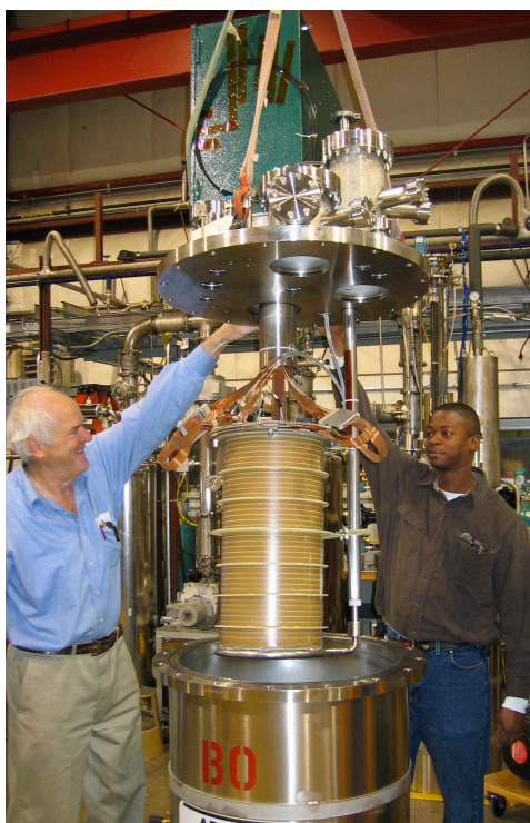
Figure 8–3: Electronics test TPC insertion into cryostat
