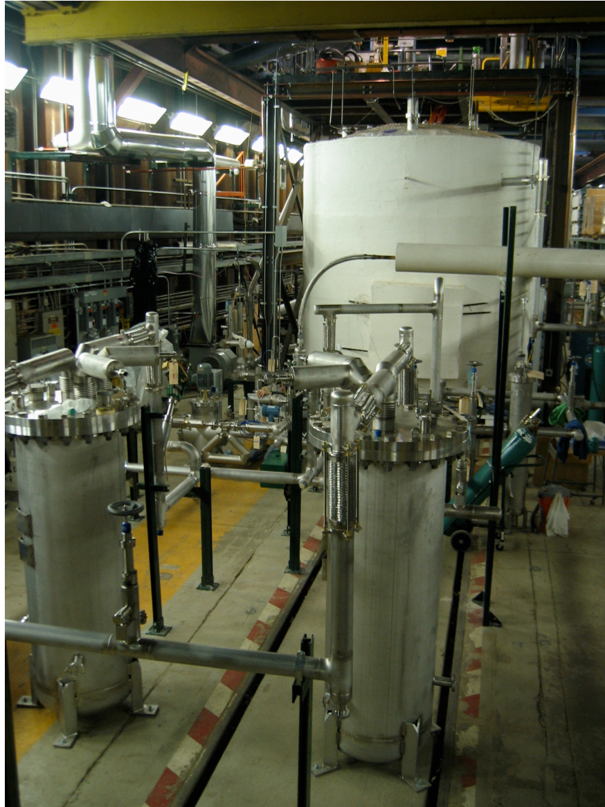
Figure 8-5: Liquid Argon Purity Demonstration filtration and tank at the PC-4 facility
