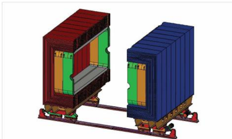
Figure 5-2: A schematic of the UA1 magnet, as used in the T2K experiment, but shown in the opened position. Interior components shown in brown, grey and green are coils. The exterior C-shapes in red and blue are magnet yokes. Both assemblies are shown on rollers and rails.
