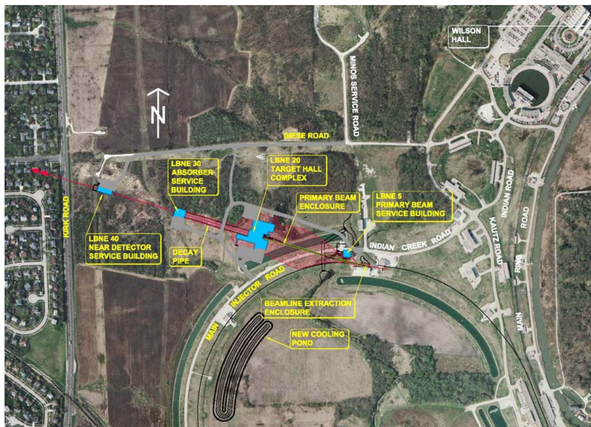
Figure 1-2: LBNE Overall Project Layout at Fermilab. Note figure orientation is shown with North at the top of the image.
