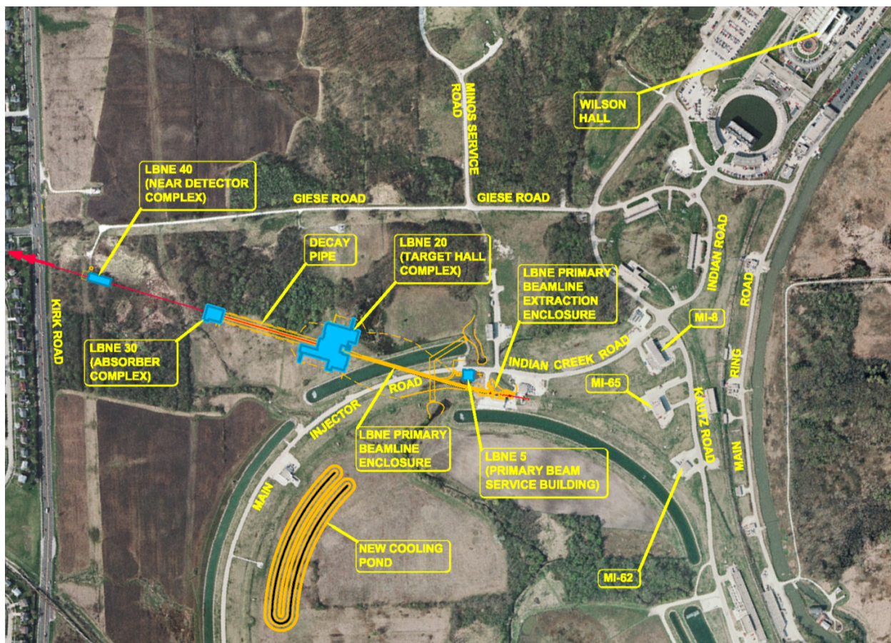
Figure 1-7: LBNE Overall Project Layout at Fermilab
