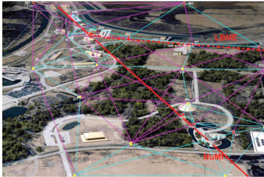
Figure 4-3: Fermilab LBNE surface geodetic network.
