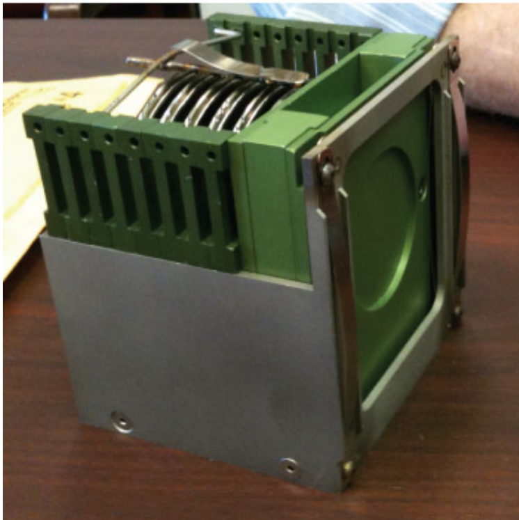
Figure 3–12: BLIP test sample holder. This figure shows cassettes of material samples irradiated in the BLIP facility. The beam enters from the right.
