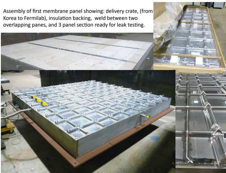
Figure 7-7: Membrane panel assembly and components
