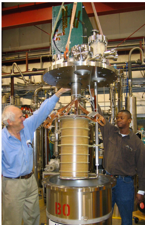
Figure 7-3: Electronics Test TPC insertion into cryostat, Bo
