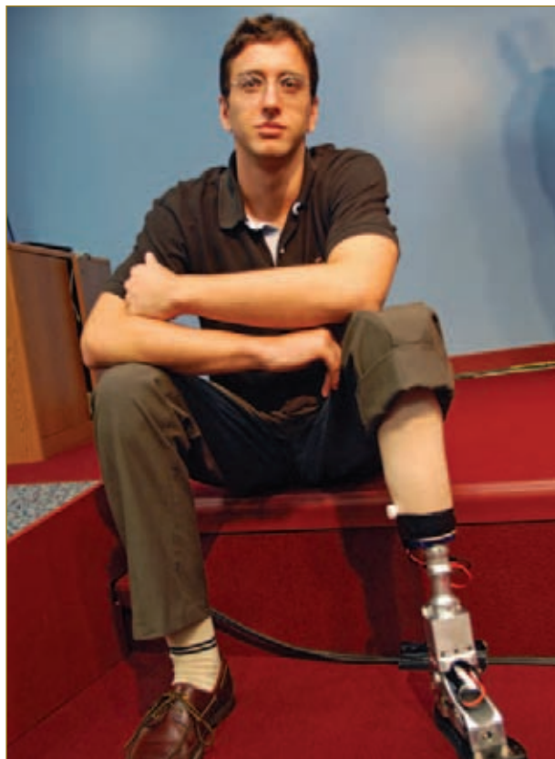
Iraq Veteran Garth Stewart helped Dr. Hugh Herr’s lab test PowerFoot, which propels users forward with tendon-like springs and an electric motor.
