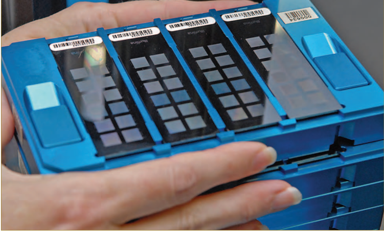
At VA's Pharmacogenomics Analysis Lab, this carrier contains slides loaded with common gene variants and DNA from research volunteers. A laser scanner will detect matches and help researchers learn which variants are linked to which health conditions. The slides are bar-coded for privacy.
