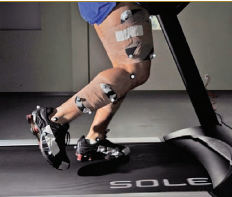
A study volunteer runs on a treadmill in the Gait and Motion Analysis Lab at the Center for Restorative and Regenerative Medicine, his legs taped with reflective markers that are tracked by motion-capture cameras. Meanwhile, researchers check the results from software that creates a 3D representation of the volunteer's leg movements.
