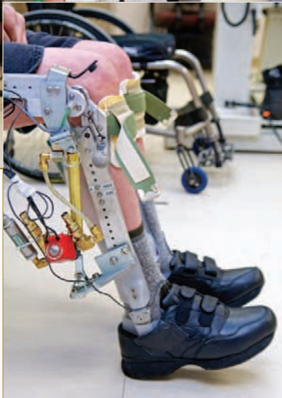
Veteran Don Crago (center) has been helping APT engineers test a dynamic brace that uses electrical stimulation to excite paralyzed muscles and controllers that lock and unlock leg joints, allowing patients to walk after full or partial paralysis. With Crago are Dr. Musa Adu, Curtis To, Rudi Kobetic and Thomas Bulea. The inset shows the brace with the knee joint in the unlocked (sitting) position.
