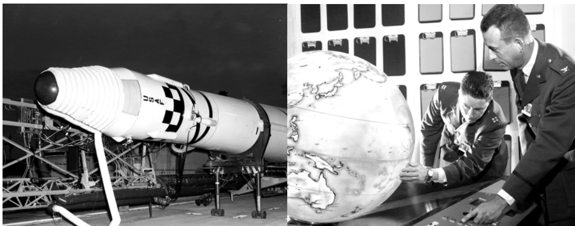
Left: The Agena spacecraft for Discoverer 13, mated to its Thor launch vehicle, waits on the pad at Vandenberg AFB before being erected. The covering cooled and protected the spacecraft. Right: Colonel C. Lee Battle, Discoverer program director, and a project officer observe the ground track of a satellite in 1960, taking care not to look at the Soviet Union.
