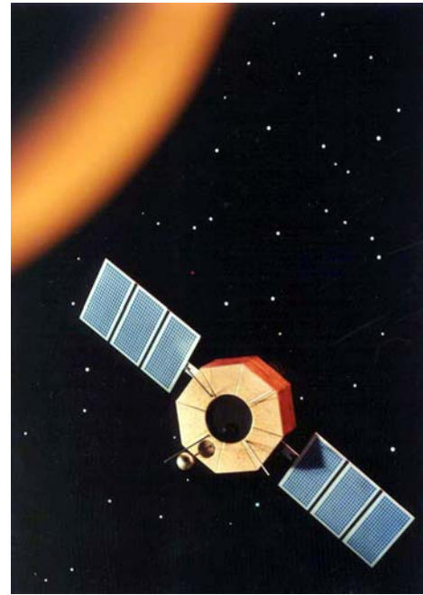
Left: The second Transit satellite (Transit 1B) undergoes checkout at Cape Canaveral before launch on 13 April 1960. Right: This artist's concept depicts the second Navigation Technology Satellite (NTS-2) in orbit. NTS-2 was used as part of the GPS Block 1 test constellation.
