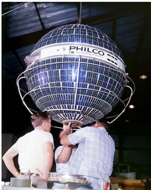
Left: The Courier 1B satellite undergoes testing at Patrick AFB before launch on 4 October 1960. Right: A conceptual model of a satellite for Project Advent. No satellite was ever actually launched for Advent.
