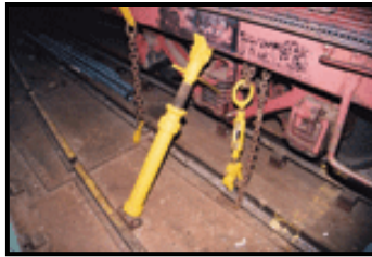
Exhibit 6-31: Railcar securement on-board a Ro/Ro vessel
