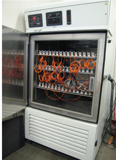
Environmental chamber burns in transducers in about 10 days.
