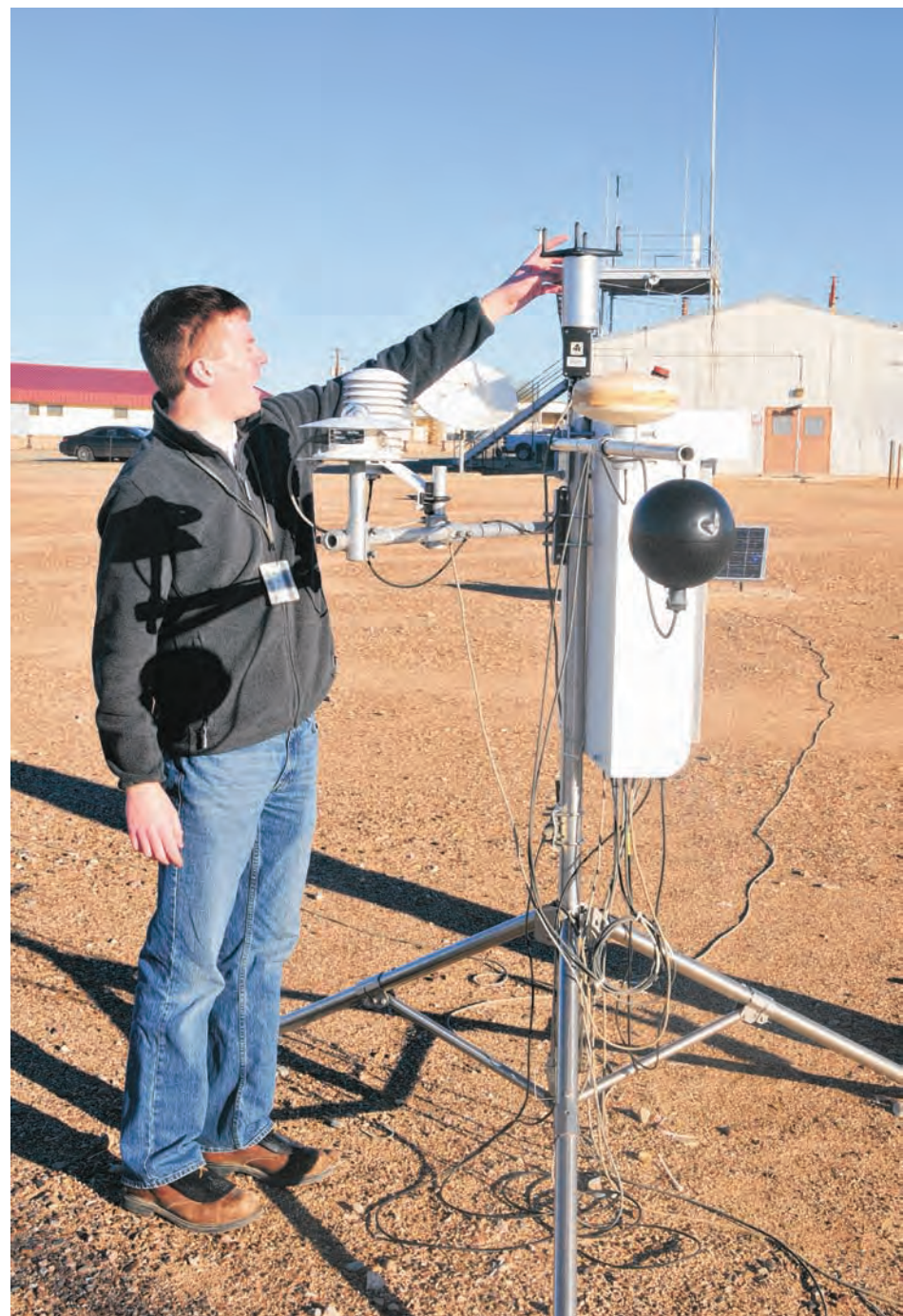
Nick McColl inspects a weather sensor platform that includes devices to measure temperature, wet bulb globe temperature, and wind speed. The team has more than 20 fixed meteorological sensor stations located across YPG's vast ranges.
