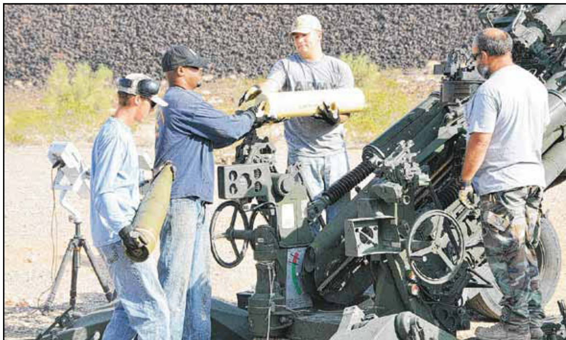
Though the proving ground's overall workload was down from its all-time high in 2011, the Munitions and Weapons Division's workload increased by about 5 percent this fiscal year. Included in this workload was the proving ground's acceptance testing of every M777 155 mm lightweight howitzer (seen here) produced prior to its being fielded to troops.
