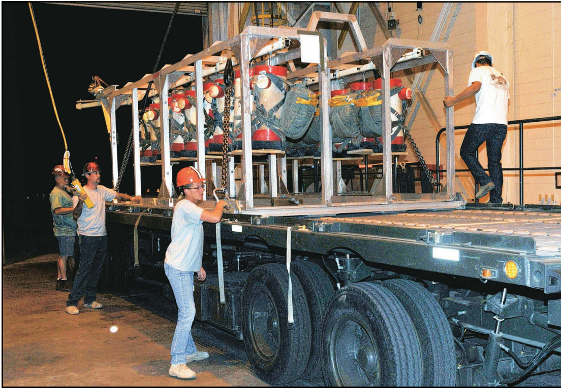
The developmental testing of the ARAPS at YPG has also included jumps with heavy, instrumented mannequins dropped from a C-130 aircraft off of a mechanically-operated rack. Here, YPG personnel load a ready-to-go rack onto a K loader prior to a test jump.
