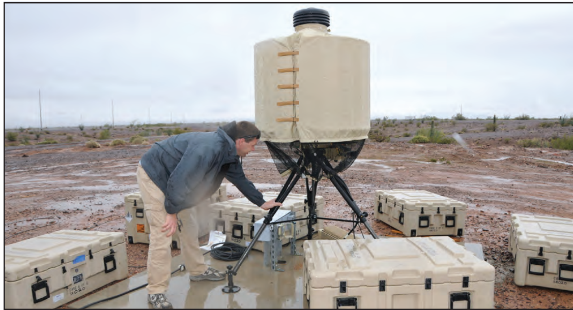
Test officer Jonny Clark inspects a Lightweight Counter Mortar Radar (LCMR) unit under evaluation at YPG. The LCMR is a groundbreaking improvement over its predecessors by providing a 360 degree detection radius for incoming rounds.
