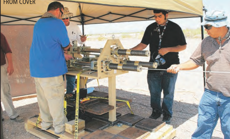
Chirag Patal (center) observes as Luis Manos (right), Charles Lott (back to camera) and Rick Guyette, prepare to do a live fire check of the .50 caliber three-barrel ballistic firing device that will be used for insensitive munitions bullet impact testing. PHOTOS BY LUCY RIVERA
