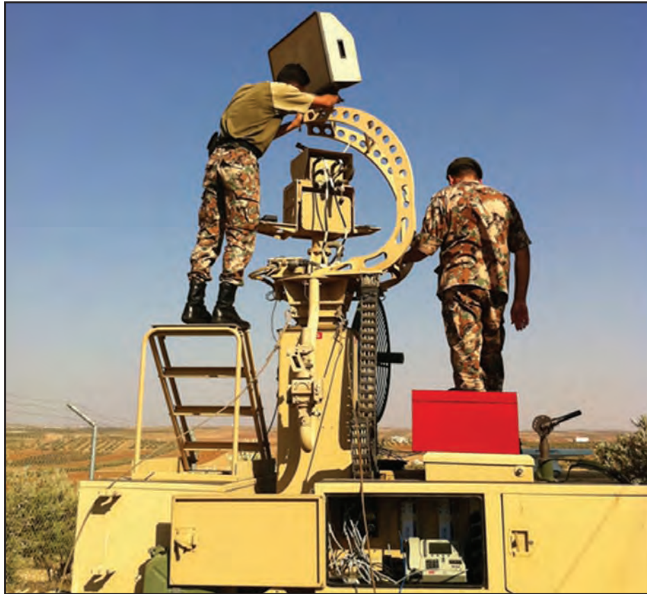
Operated by Jordanian soldiers on a 50 kilometer section of its border, the YPG-tested "virtual fence" includes a wide variety of equipment used to detect vehicles and people crossing the border.
