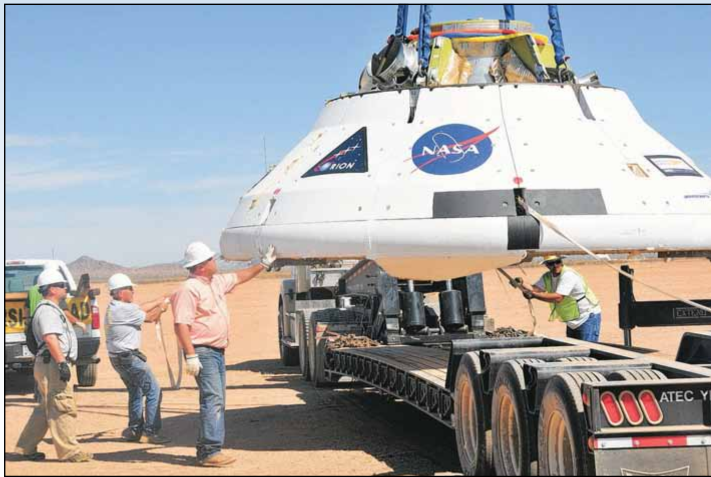
Though the drop test article is smaller than the actual Orion capsule, it still requires a large crane to lift. Here, the mock capsule is carefully maneuvered onto a low boy trailer from YPG's motor pool after the test drop.
