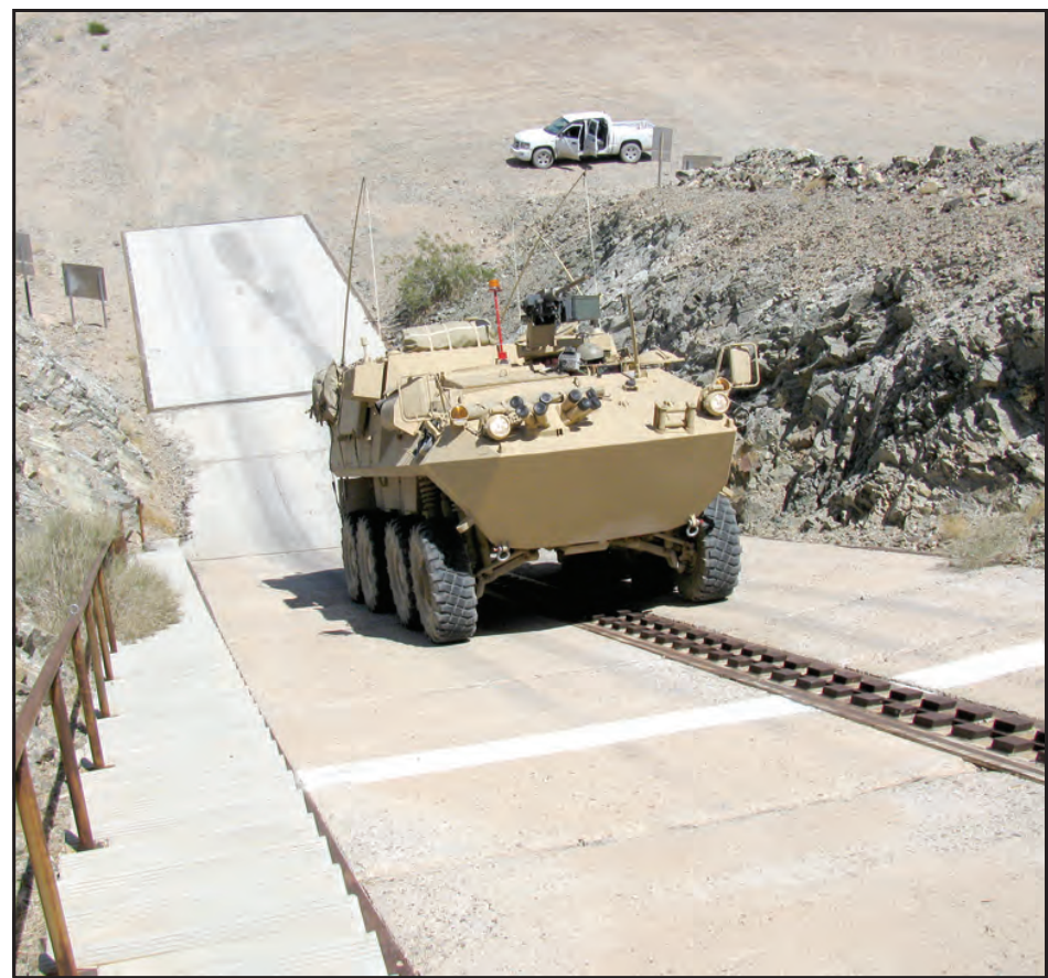
The Light Armored Vehicle (LAV) and its variants have served the US Marine Corps and friendly foreign nations for more than 25 years. Here, a LAV under test for a foreign customer is tested on one of YPG's 60 percent grades as part of a comprehensive endurance evaluation.
