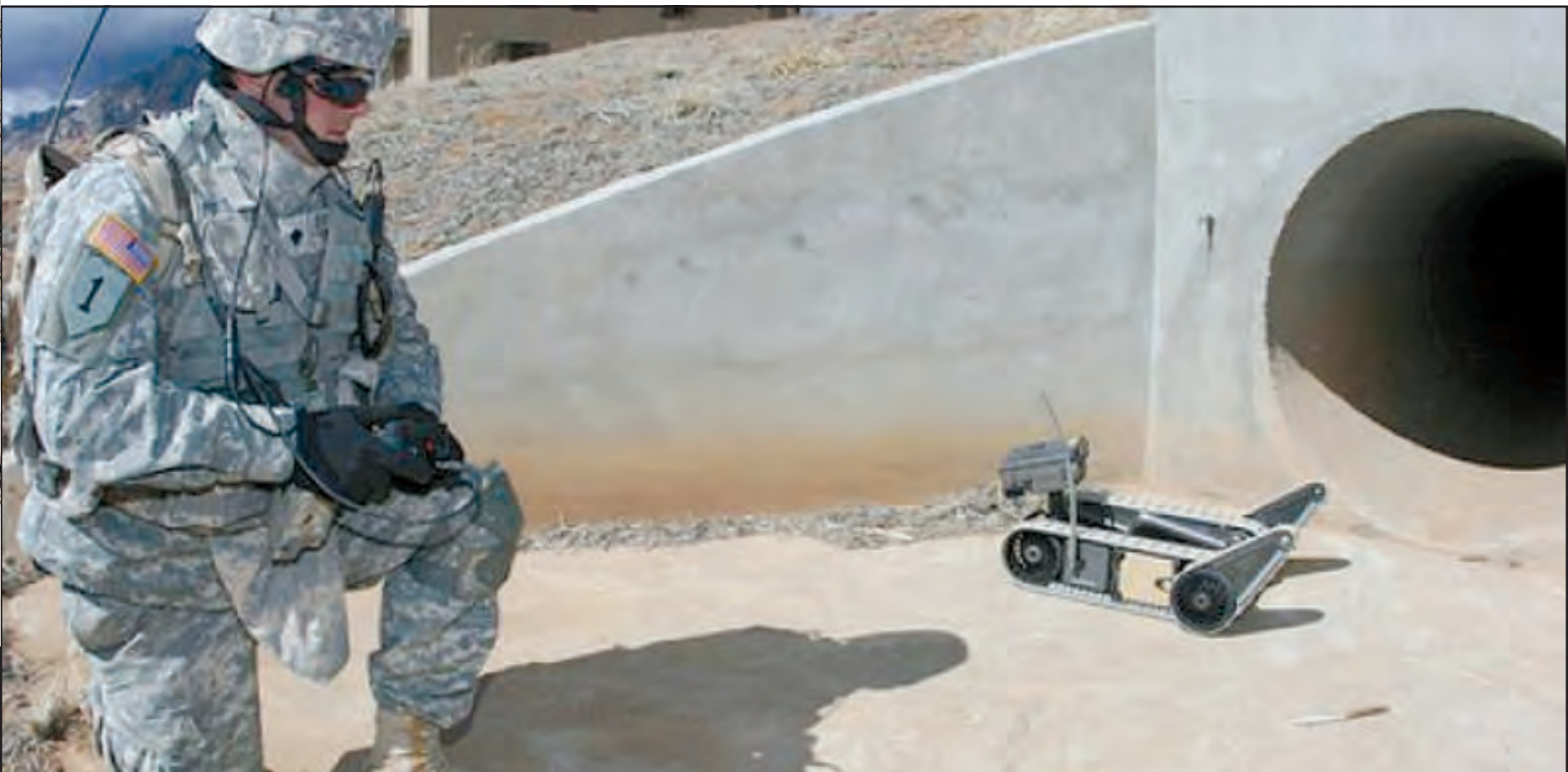
A Soldier at Fort Bliss, Texas, prepares to use an unmanned ground vehicle to search a tunnel. The tunnel could hold unseen dangers and it's better to lose a piece of machinery than a human life.
