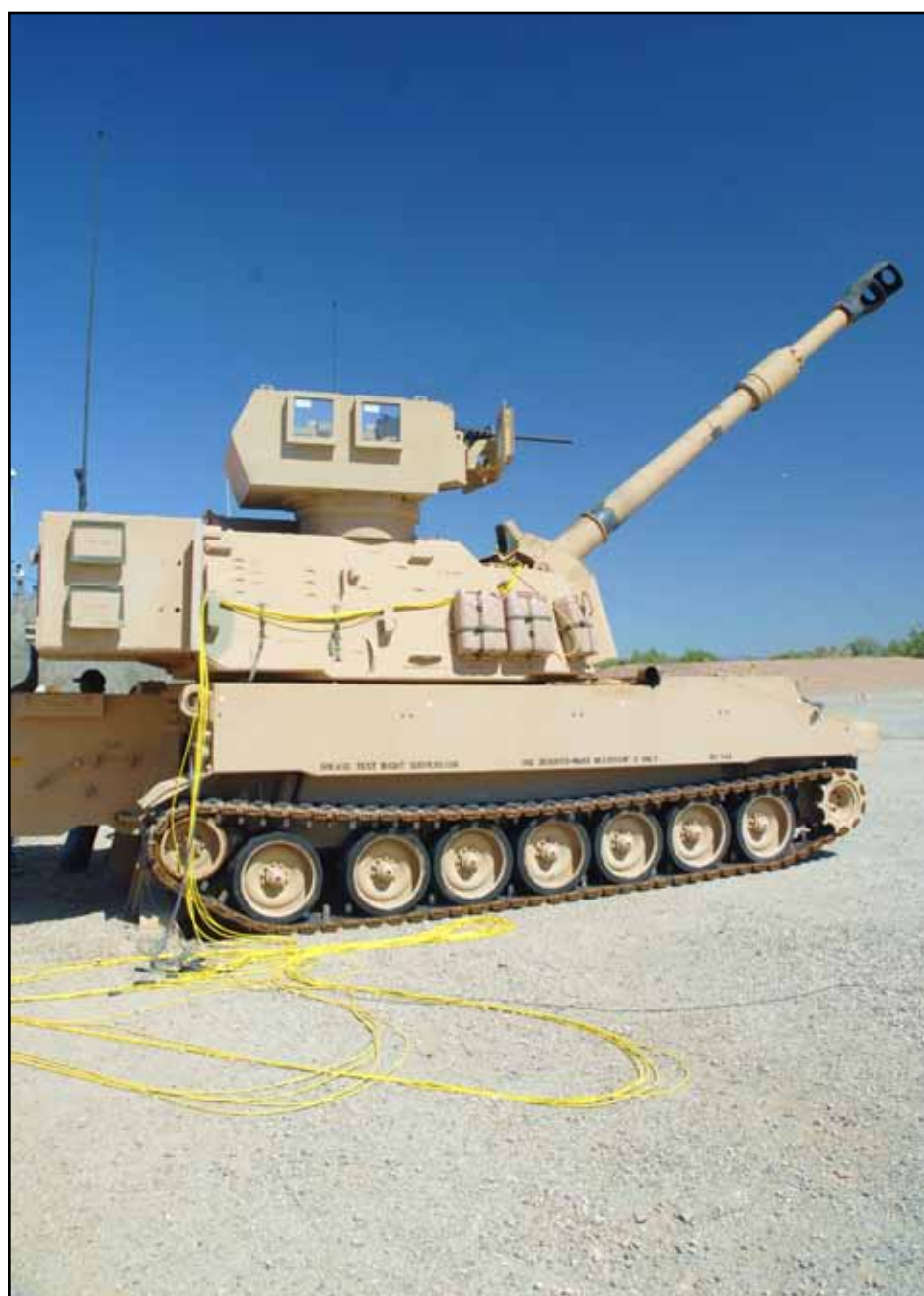
Projectiles fired by the M109A6 Paladin self-propelled howitzer weigh more than 100 pounds and its range is achieved by adding propelling charges. The weight of the ammo didn't slow the quick action of the gunners when nearby sparking threatened a 'cook off': "In an instant, one gun crew member had a fire extinguisher," recalled test officer Mike Dickerson. "The gun crew leader actually walked the 100 pound bullet all the way back behind the conditioning chamber, which is behind a reinforced concrete wall, and another gunner walked the charge back." (Loaned photo)
