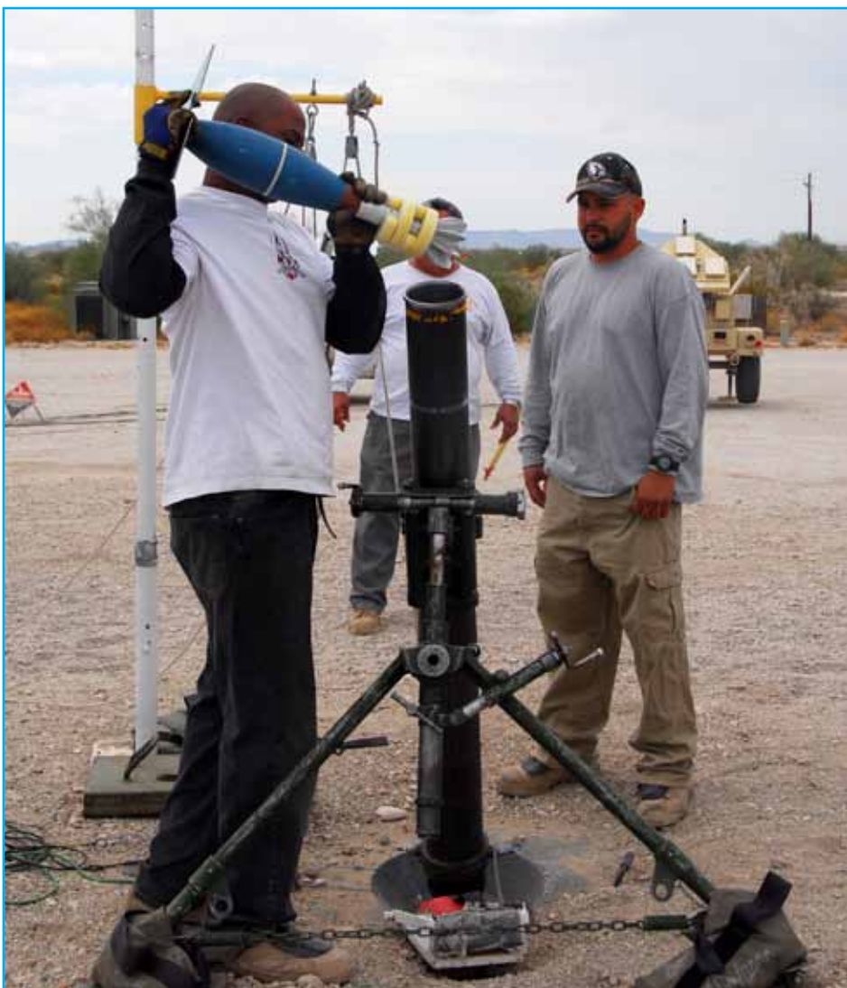
Weapons operator Thomas Brown loads the guided 120 mm mortar projectile. The advanced initiative to field a guided mortar round to troops meant heavy testing of the projectile at YPG for nearly a year.
