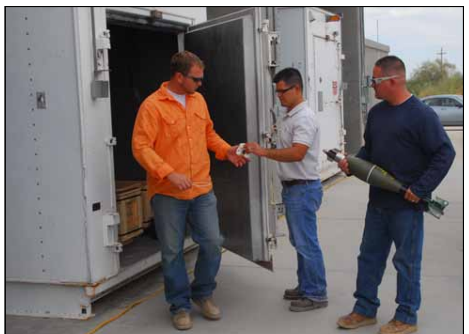
Developmental testers usually want to see how their system can perform when conditioned to temperatures as low as -50 degrees and as high as 145 degrees, and YPG has conditioning chambers to accomplish this all year round. Here, test officer Arturo Anaya (center) and Pedro Bayanas (right) remove an APMI round from a conditioning chamber.
