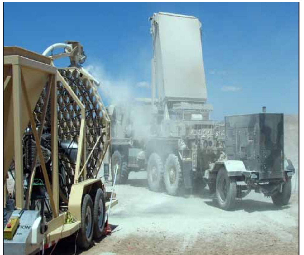
The Blowing Air Dust and Sand System developed by YPG personnel is critical to testing equipment's survivability in desert conditions. (Loaned photo)
