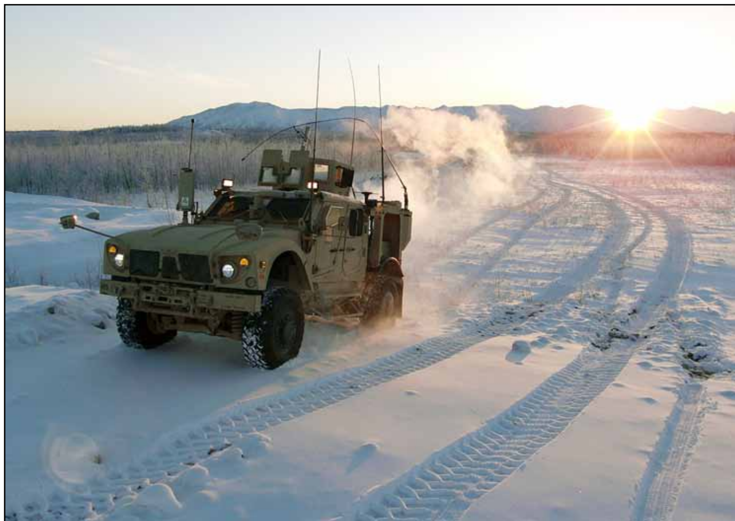
Lighter and more maneuverable than prior Mine Resistant Ambush Protected (MRAP) vehicles, the MRAP-All Terrain Vehicle (M-ATV) is currently undergoing rigorous testing at Cold Regions Test Center after seeing extensive evaluation at Yuma Test Center. Soldiers from the 6th Engineer Battalion, United States Army Alaska, are serving as test participants. (Photo by Mike Kingston)
