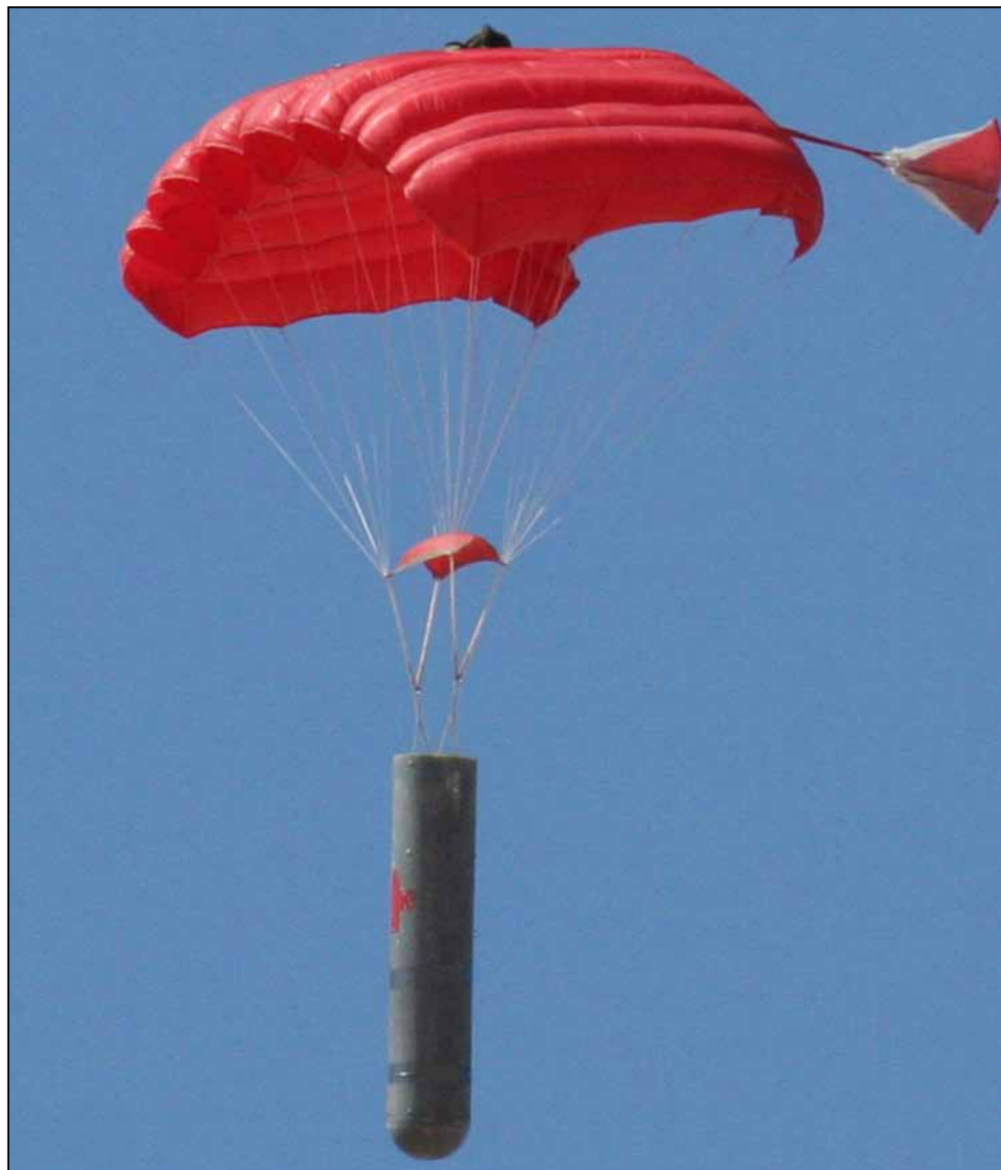
The Provider supply pod can carry supplies from blood transfusions to vaccines, be re-used as many as 30 times, and be packed and rigged in a matter of hours by personnel with only a few days of training. Here, the pod is steered into a soft landing by a guided parachute that is part of the JMDSE test program. (Loaned photo)
