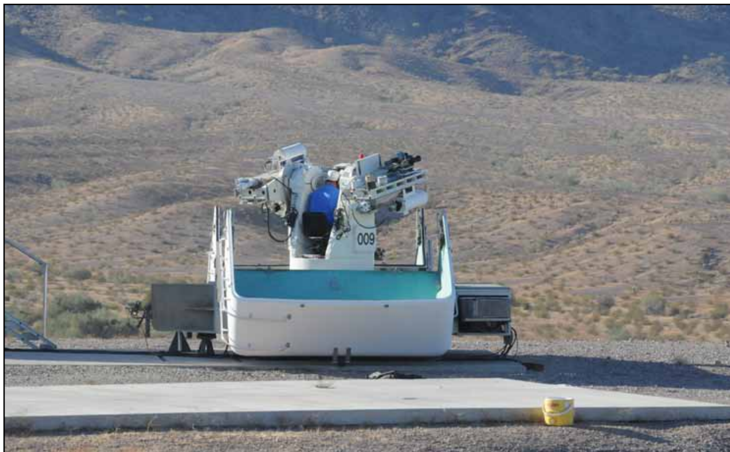
Tracking the flight of tiny pods dropped from unmanned aircraft at altitudes as high as 25,000 feet is accomplished with sophisticated tracking mounts like the one seen here. "If you go somewhere other than YPG, the riggers, test officers and equipment aren't available, so you would have to build them up," said project officer Sanjay Patel. "Coming here allows us to focus exclusively on the test." (Photo by Mark Schauer)
