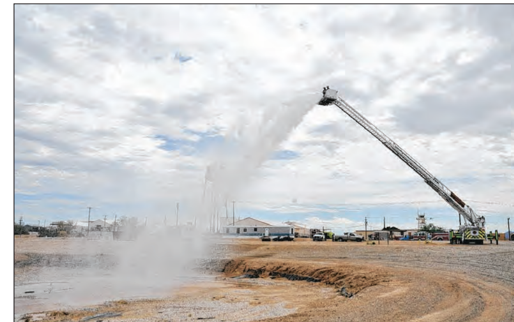
The new truck's platform also has an attached hose that can be operated by firefighters on the platform itself or from the truck, which allows the department to attack fires from high above with up to 2,000 gallons of water per minute.
