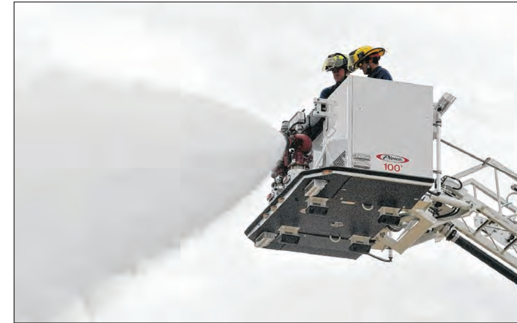
Though its ladder is the same length as its 20 year-old predecessor, the new truck boasts significant capability and safety improvements, including the aerial platform at the end of the ladder that can quickly raise firefighters high above a conflagration, as seen here.
