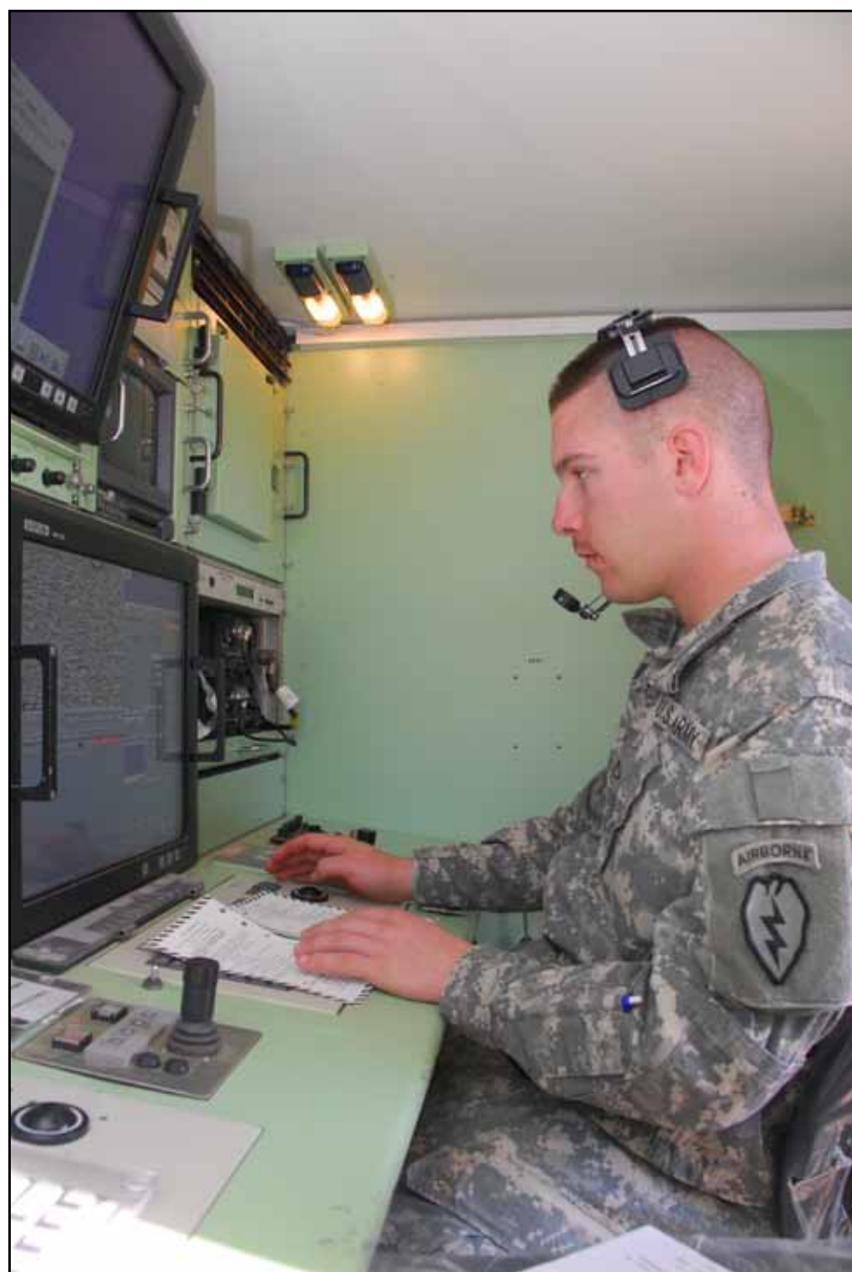
During the training, Soldiers control the Shadow and its camera from a ground control station just as they would in theater. The Shadow can loiter over an area for hours, providing intelligence to a unit commander.
