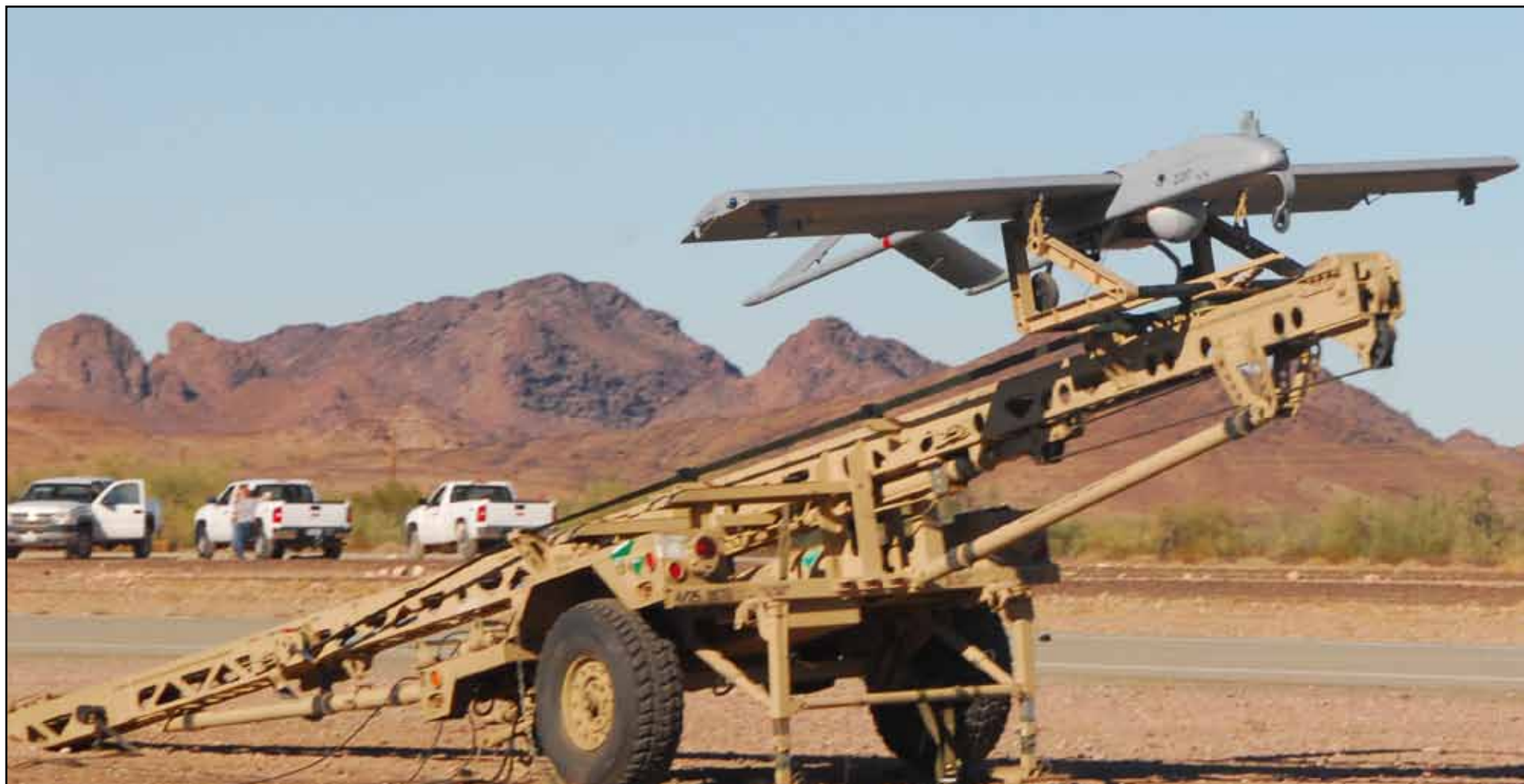
The Shadow UAS is launched off a trailer-mounted catapult that pneumatically accelerates the 400-pound craft down a long steel rail from a standstill to 65 miles per hour in a split second. “Our unit needs to keep current in its training, and another warrant officer recommended Yuma for its air space and weather,” said Chief Warrant Officer Nicholas Jones. “Yuma Proving Ground made it so easy, we ended up coming.”
