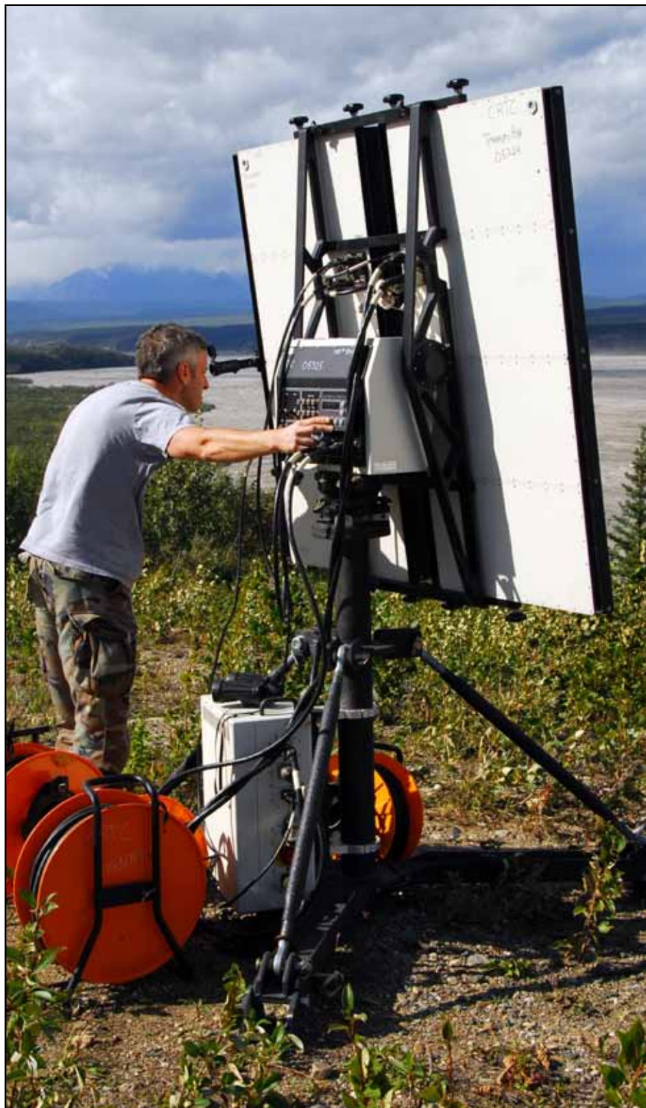
Accurate data is important in every test, and summer is an ideal time to recalibrate CRTC's sophisticated equipment after a harsh winter of use. Here, instrumentation engineer Dan Fox calibrates a Doppler radar system used in missile tests. "This would be possible in winter, but much more difficult," Fox said. (Photos by Mark Schauer)
