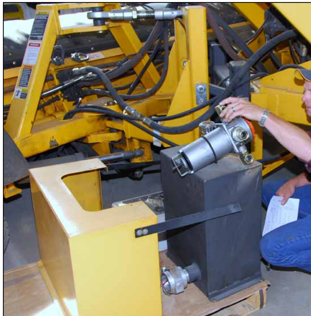
Maintenance chief Todd Zachgo inspects the hydraulic displacement pump and other mechanics are responsible for the upkeep of CRTC's fleet of over 40 wheeled and tracked generators used on remote parts of the range.
