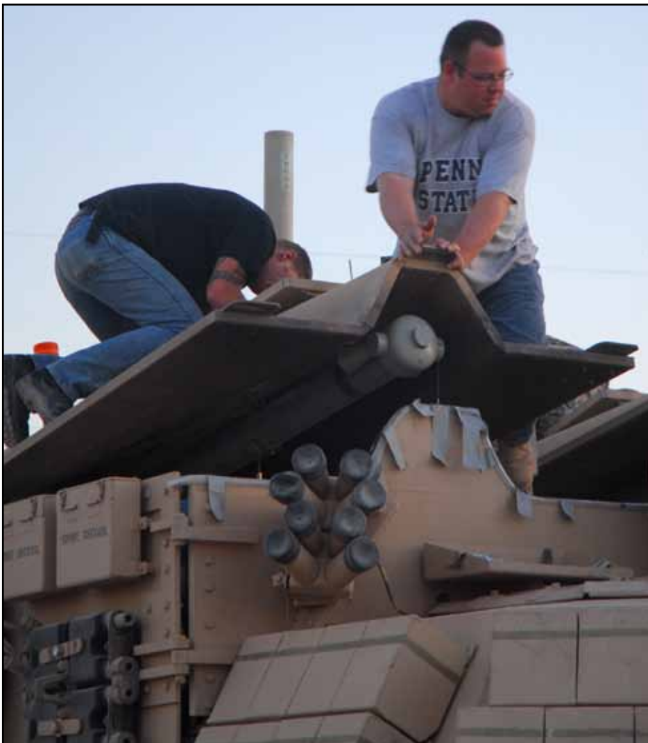
The Assault Breacher Vehicle (ABV) uses 350-foot long rocket-launched cords packed with nearly a ton of C4 plastic explosive each to detonate mines or IEDs in its path. Safely loading the heavy charges prior to testing is a painstaking process. (Photo by Mark Schauer)
