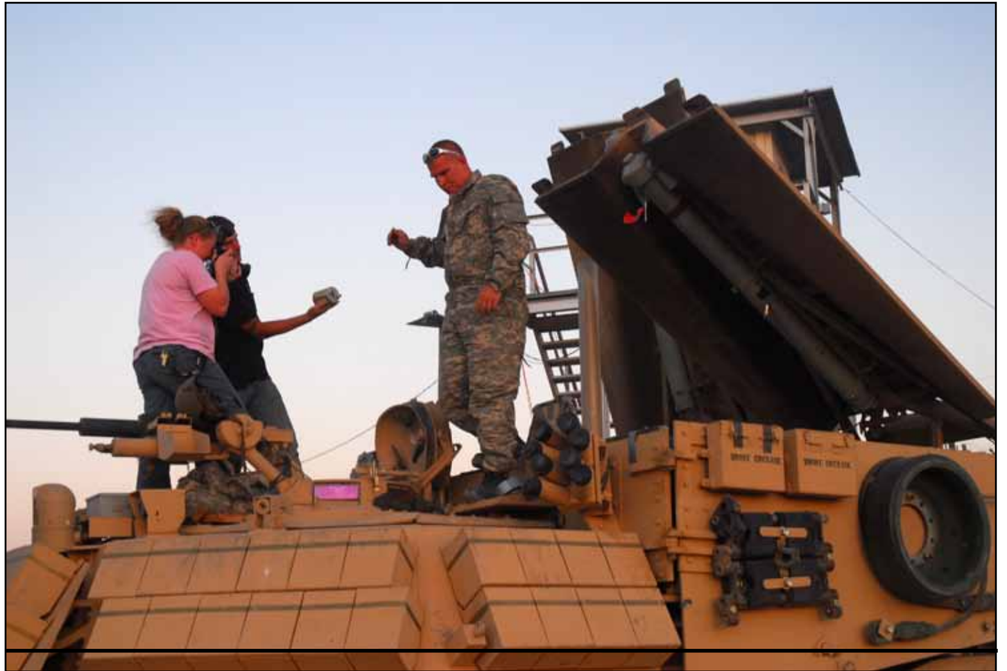
With the Linear Demolition Charge System locked and loaded, the ABV is ready for test firing. YPG’s vast test ranges and flexible workforce allow this highly specialized vehicle to be rapidly and safely tested. (Photos by Mark Schauer)
